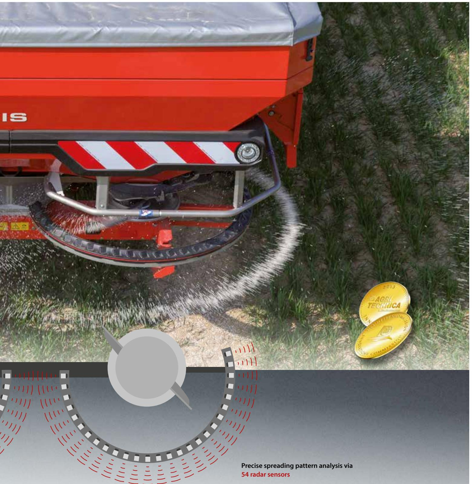
Precise spreading pattern analysis via
