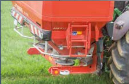
AXIS H – Right and left edge spreading via rotation speed and drop point adjustment
