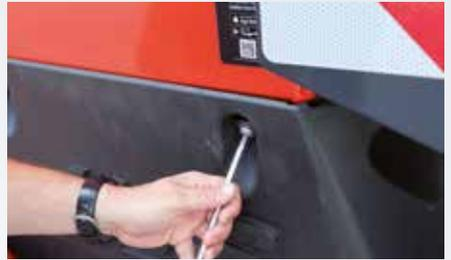
Dirt deflector with quick release fastener
