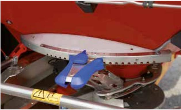
The easily readable, quantity-proportional DfC scale, unique to RAUCH, allows reliable quantity corrections after a calibration run.
