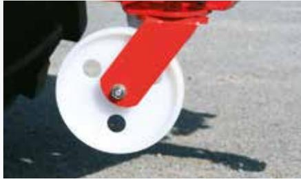
Parking rollers with quick release coupling system
