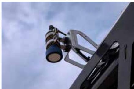
Distance Control: Ultraschallsensor
