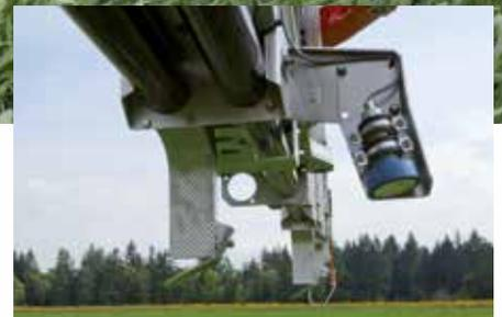
Distance Control: Ultraschallsensor
