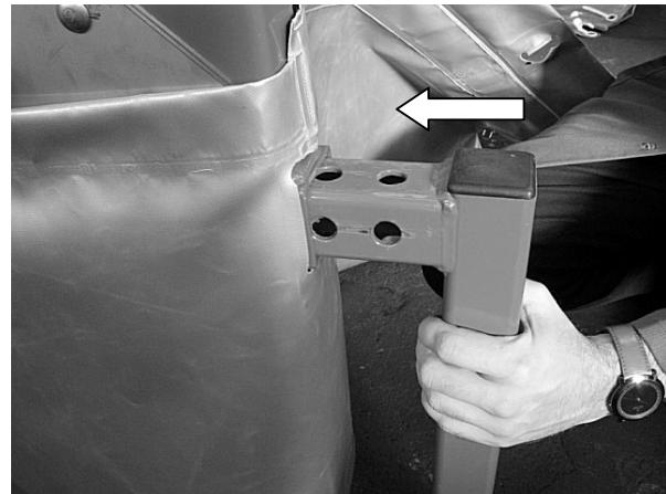
9. Screw the cover to the brackets on the frame tube on the hitch side with the star screw (3) (see picture).
