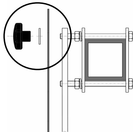
10. Pull out the **left** support foot in the hitch side (in the direction of travel for rear hitch) and slide it through **hole 2** of the cover on the spreader.
