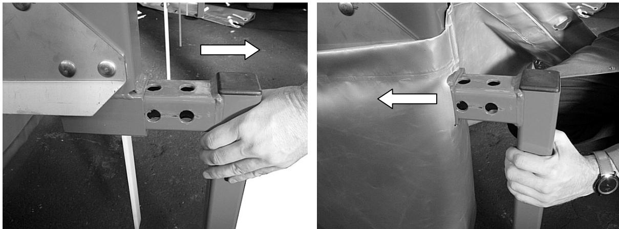
14. Attach the cover to the star screws on the folding spreader floor.
