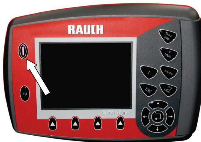
12.10. **Disconnect the QUANTRON-A** from the power supply and from the spreader.
