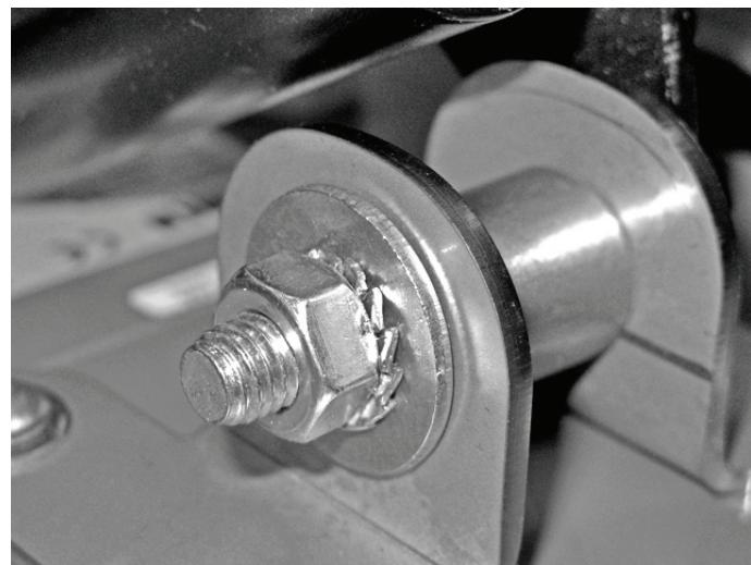
08.5. Tighten the lens head screws at the second retaining plate.
