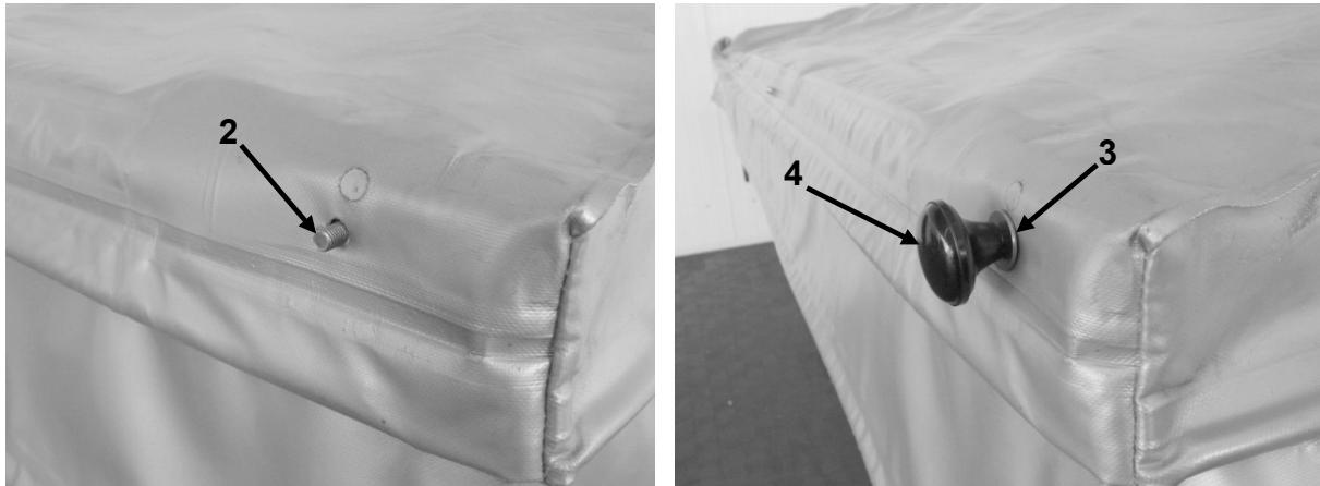
11. Bolt the round headed studs (used to attach the rubber straps) into place using the corresponding bolts, black synthetic washers, washers and nuts on both sides of the spreader.
