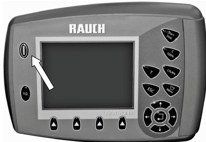
11.9. Disconnect the QUANTRON-A from the voltage supply.
