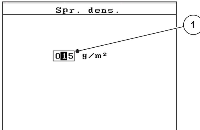
**Figure 4.29:** Input of numerical value (example spreading density)
