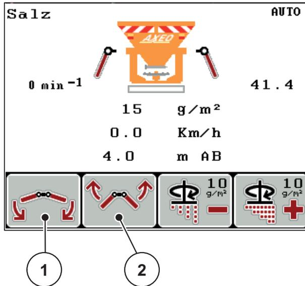
**Figure 5.3:** Spreading width adjustment with levers
