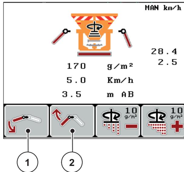
**Figure 5.6:** Asymmetric spreading pattern (example)
