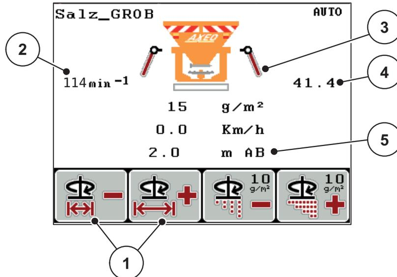
**Figure 5.8:** Working width adjustment (Dispersion AUTO function activated)
