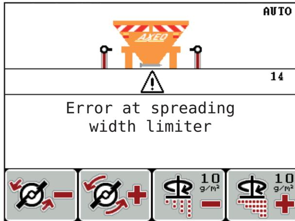
**Figure 6.1:** Alarm message (example: spreading width limiter)
