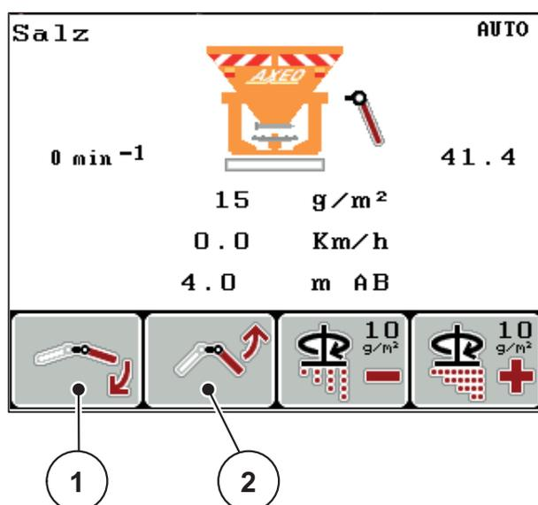
**Figure 5.2:** Spreading width adjustment with one actuator
