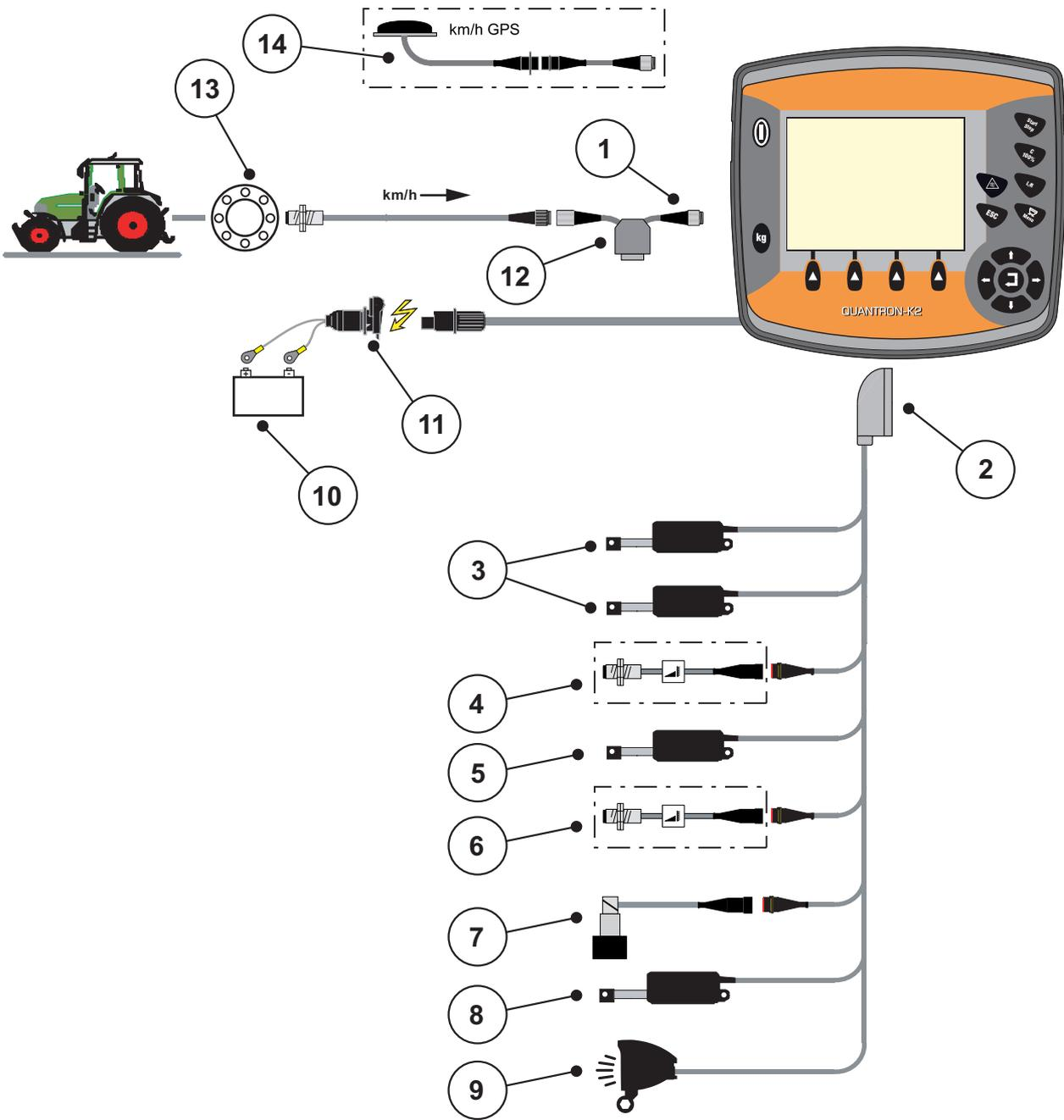
Figure 3.4: Schematic connection diagram QUANTRON-K2 (wheel sensor)
