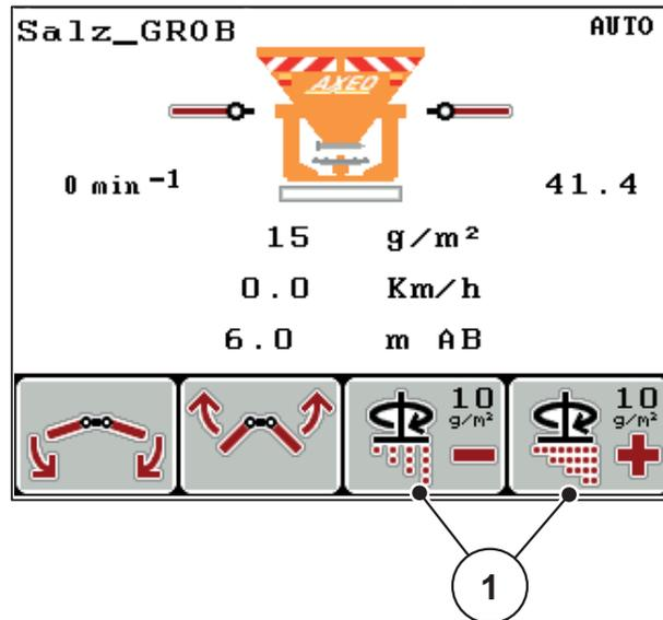
Figure 5.13: Spreading density adjustment
