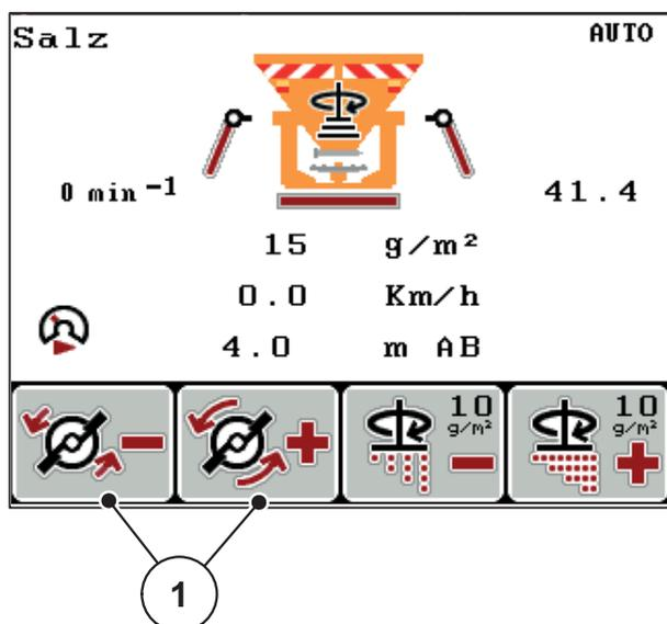
**Figure 5.14:** Disc speed adjustment
