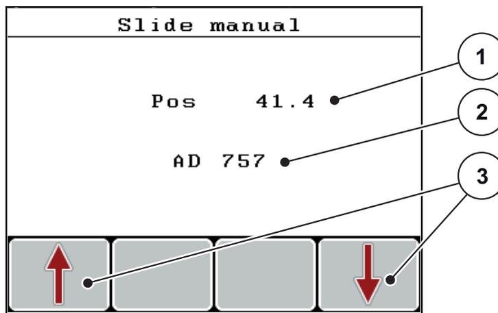
**Figure 4.26:** Test/diagnostics; example: Metering slide
