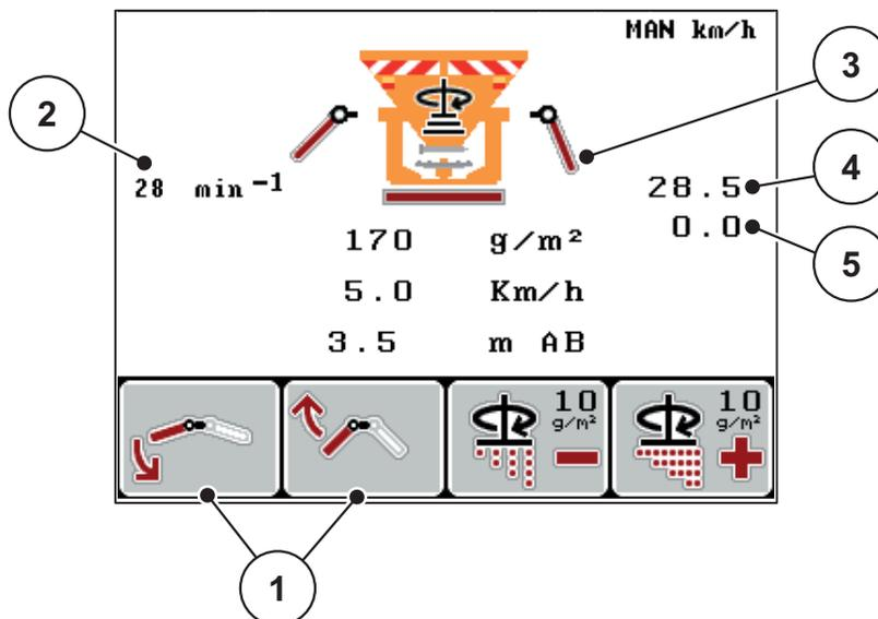
Figure 5.9: Working width adjustment (Dispersion AUTO function activated)
