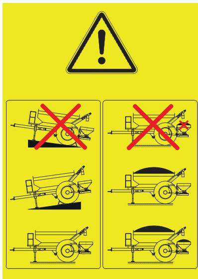
**Figure 7.5:** Warning sticker for parking the load transfer vehicle TWS 85.1
