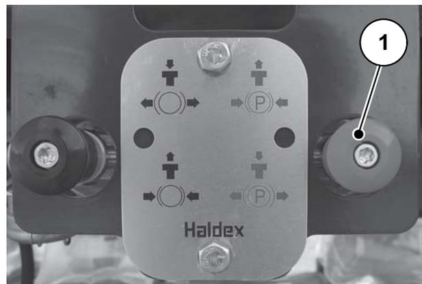
1. Press in the valve [1] for releasing the parking brake.
