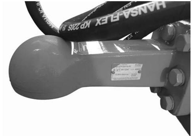
**Figure 9.15:** Ball coupling
