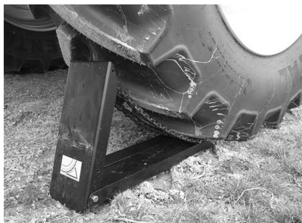
**Figure 7.8:** Position the wheel chock
