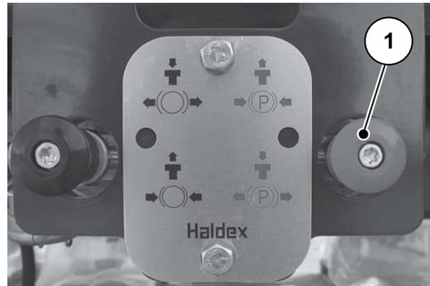
**Figure 7.6:** Apply the parking brake
