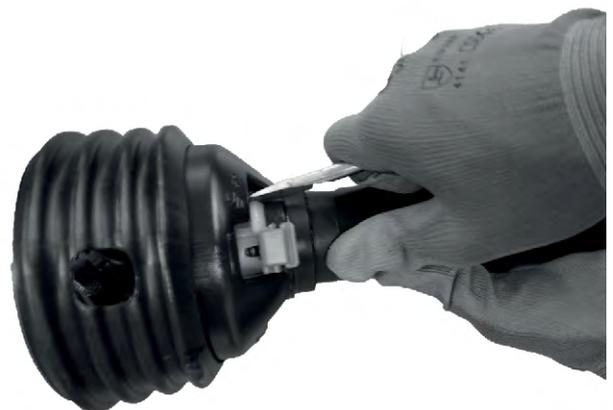
*Fig. 11: Opening the universal drive shaft cover*
