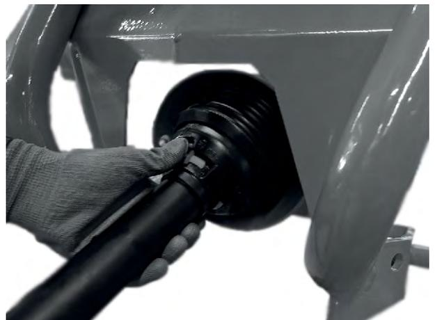
*Fig. 14: Mounting the universal drive shaft cover*
