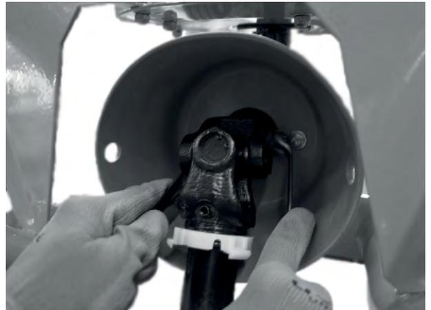
*Fig. 13: Connecting the universal drive shaft*
