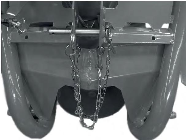
Fig. 15: Secured pin
