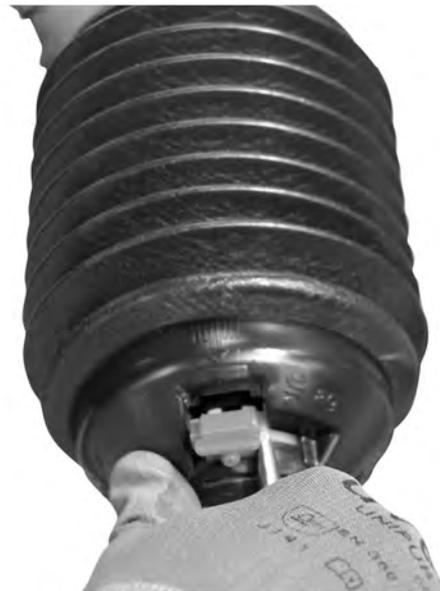
*Fig. 13: Opening the universal drive shaft guard*
