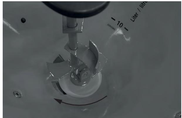
Fig. 37: Hopper without protective grid
