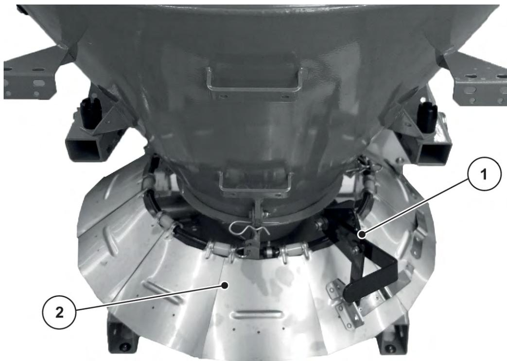
*Fig. 26: Spreading width limiter setting*
