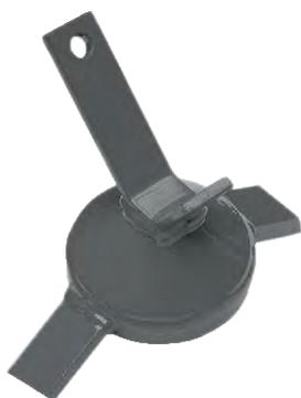
Fig. 9: Agitator for granular fertilizer
