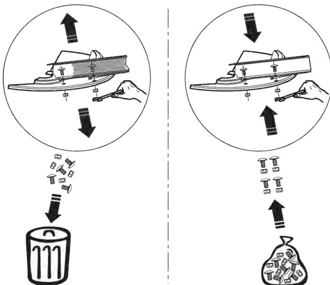
Fig. 36: Using new self-locking nuts
