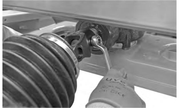
*Fig. 15: Connecting the universal drive shaft*
