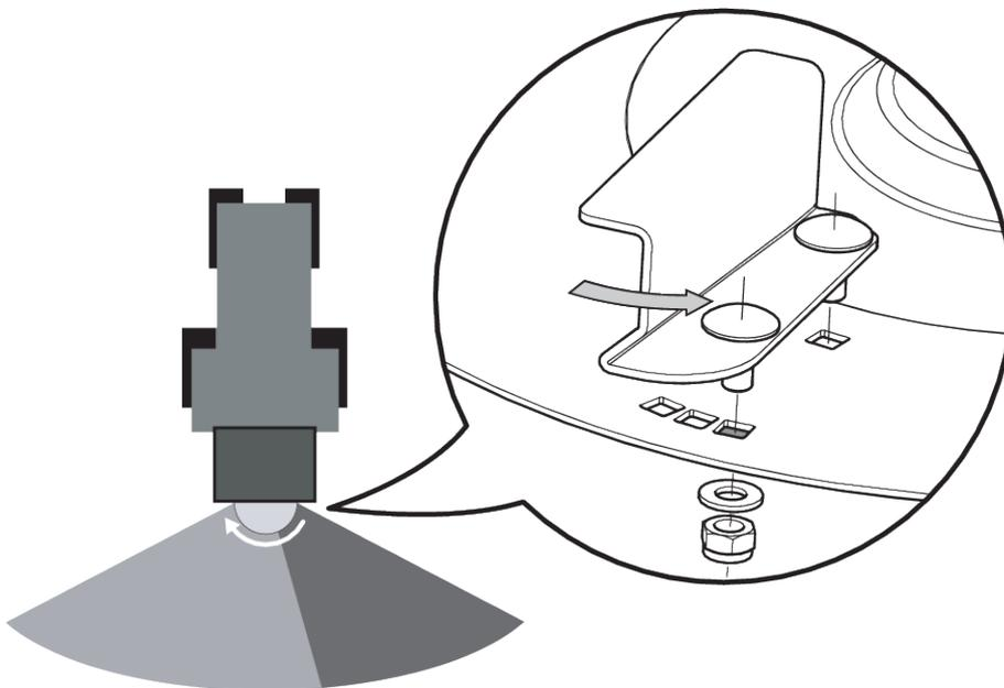
Fig. 22: Spreading density on the right in direction of travel
