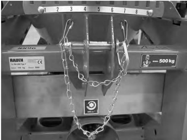
Fig. 18: Secured pin
