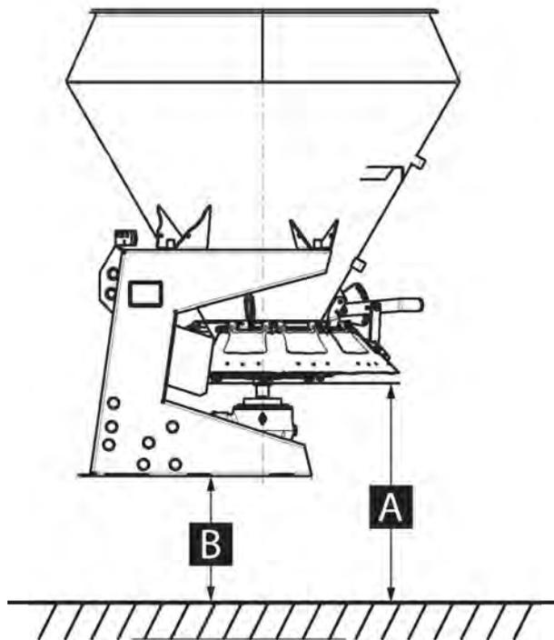
Fig. 19: Setting the mounting height
