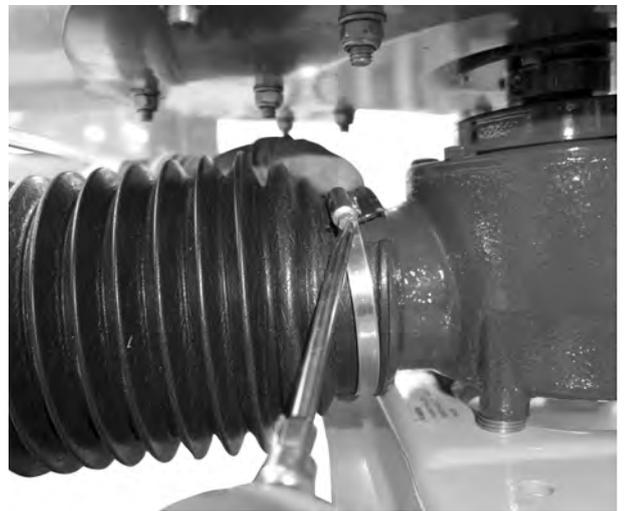
*Fig. 16: Mounting the universal drive shaft guard*
