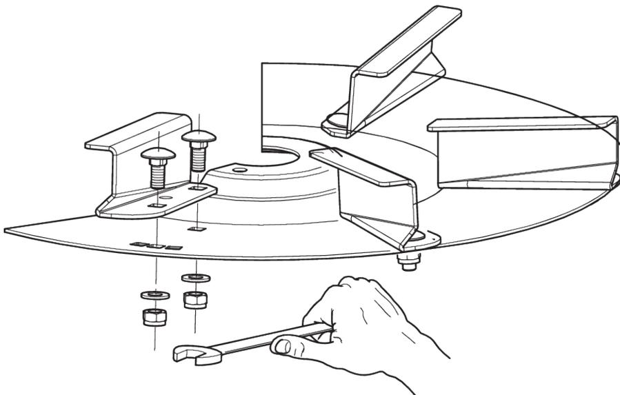
Fig. 35: Loosening the screws of the spreading vane
