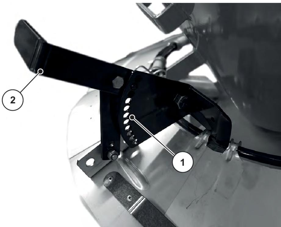
*Fig. 30: Spreading width limiter*
