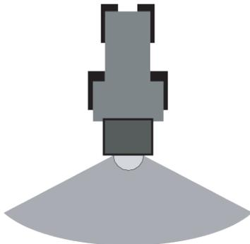
Fig. 28: Symmetrical spreading pattern
