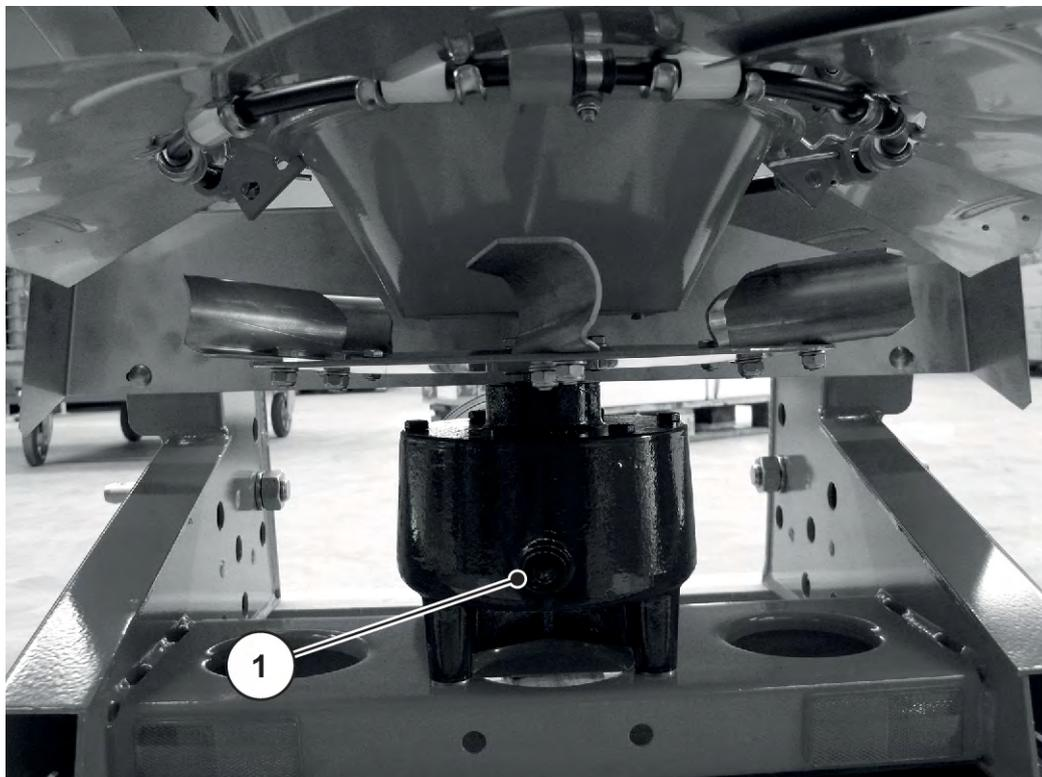
Fig. 39: Transmission oil level checking screw
