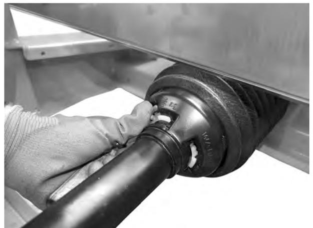
*Fig. 17: Securing the universal drive shaft cover*
