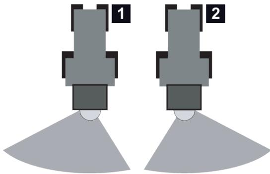
Fig. 29: Asymmetrical spreading pattern
