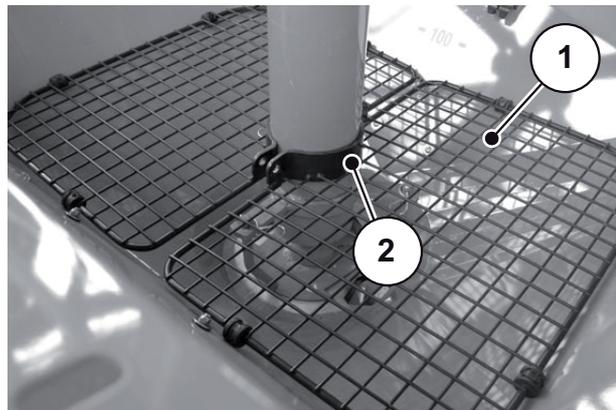
Figure 5.13: Protective grid in hopper
