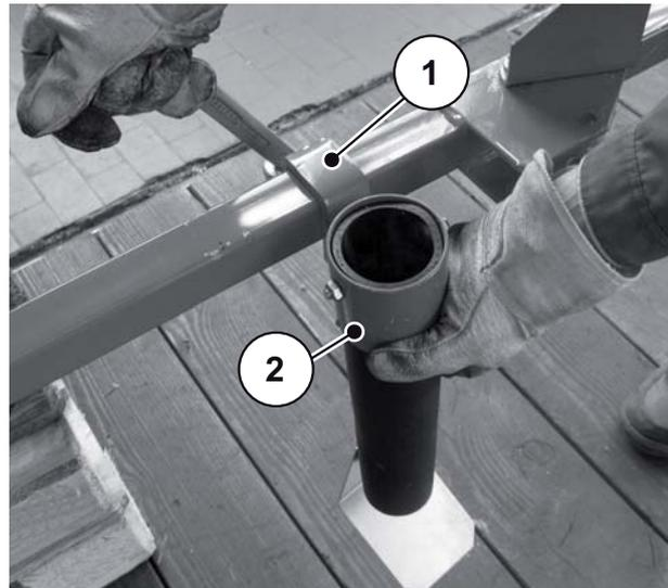
Figure 5.24: Assemble outlet pipes
