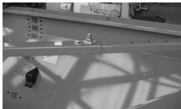
**Figure 5.15:** Fasten the centre part of the strut.
