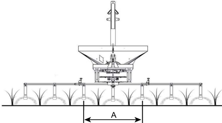
**Figure 6.2:** Spreading with baffle plate
