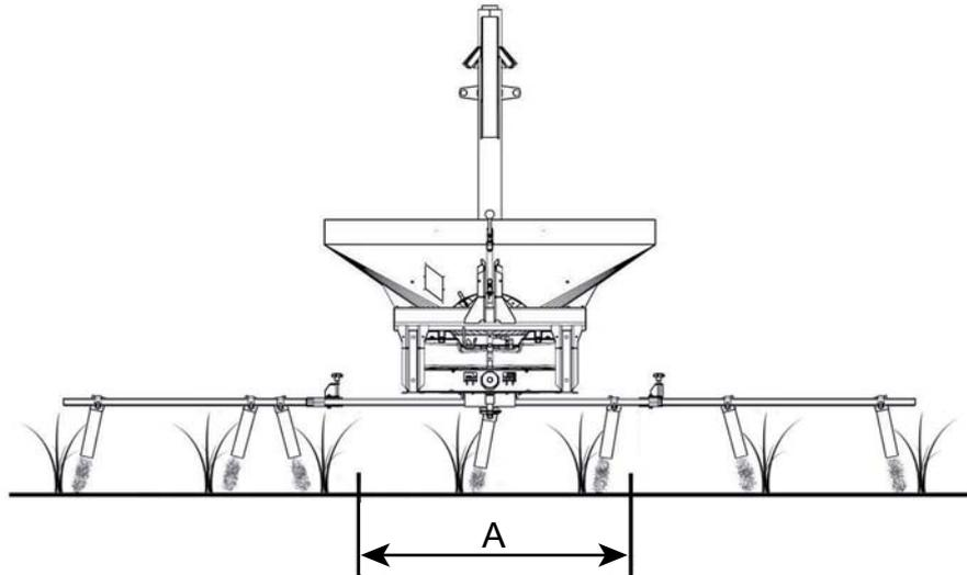
**Figure 6.3:** Spreading without baffle plate
