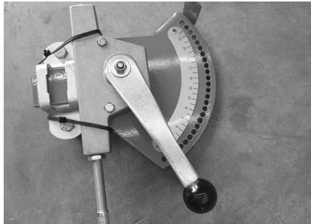
**Figure 5.26:** Metering slide actuator
