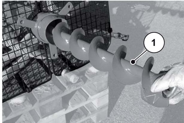
Figure 9.7: Pull out the screw conveyor
