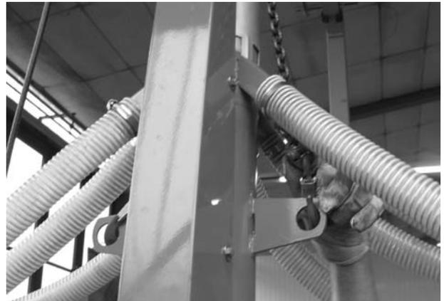
**Figure 9.1:** Attach the lifting gear to the screw tube
