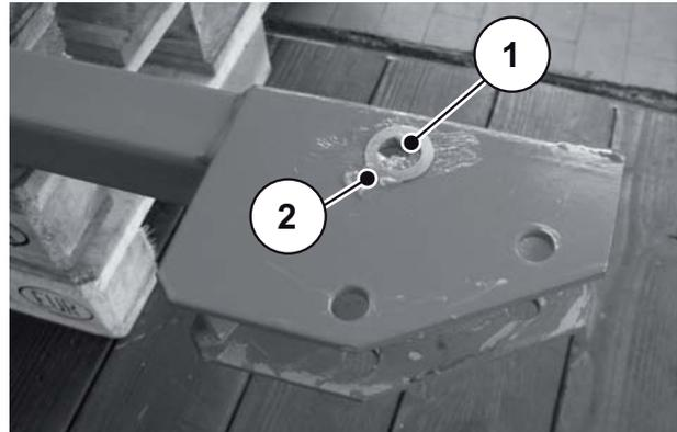
**Figure 5.19:** Place adjusting washer
