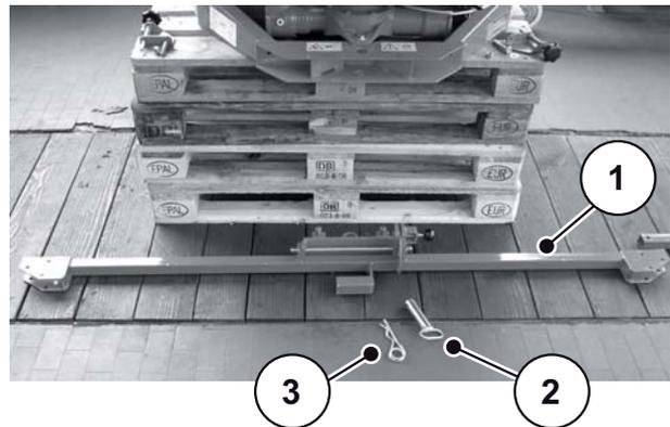
Figure 5.16: Central part and components
