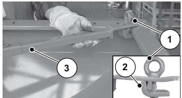
**Figure 9.2:** Loosen the adjustable struts.
