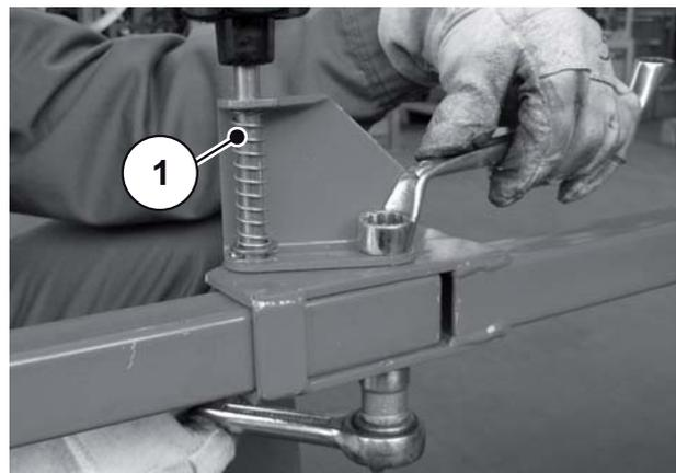
**Figure 5.20:** Lock mechanism between side and central part
