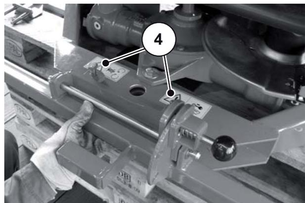
Figure 5.17: Attach the central part
