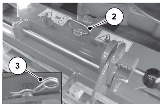
Figure 5.18: Secure the central part with the plug
