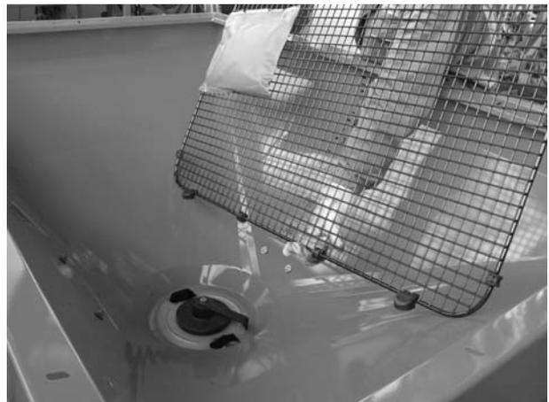
Figure 5.3: Remove the protective grid
