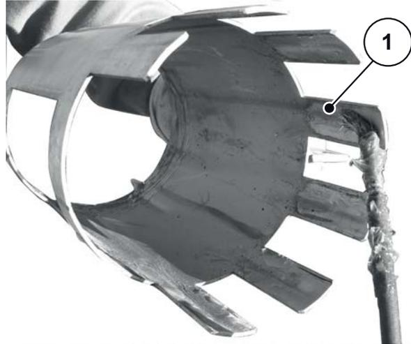
5. Lubricate the inner side of the slide sprockets.
