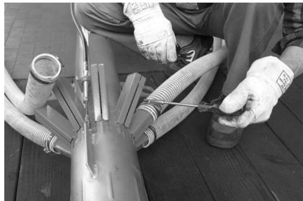
**Figure 5.7:** Tighten the hose clamps
