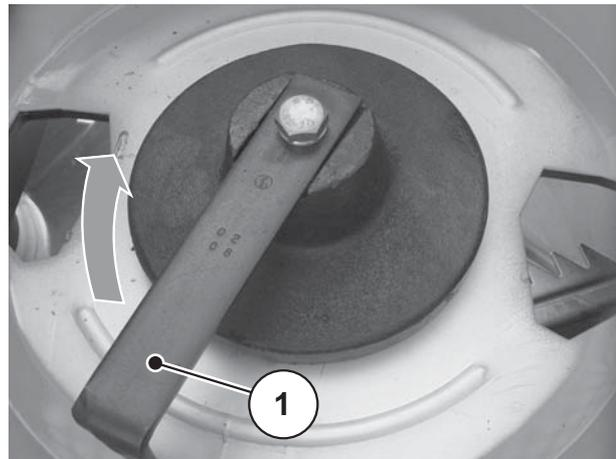
Figure 5.4: Remove the agitator
