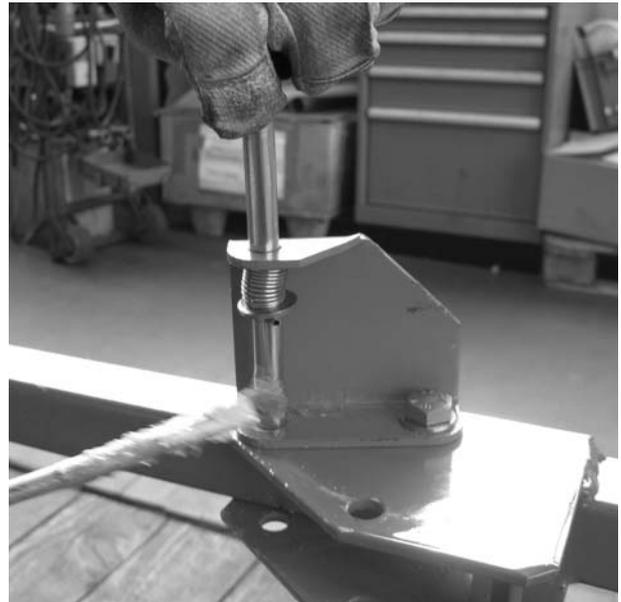
**Figure 5.21:** Lubricate the lock mechanism
