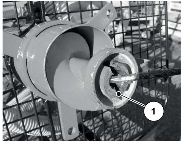
Figure 9.10:Socket of the screw conveyor
