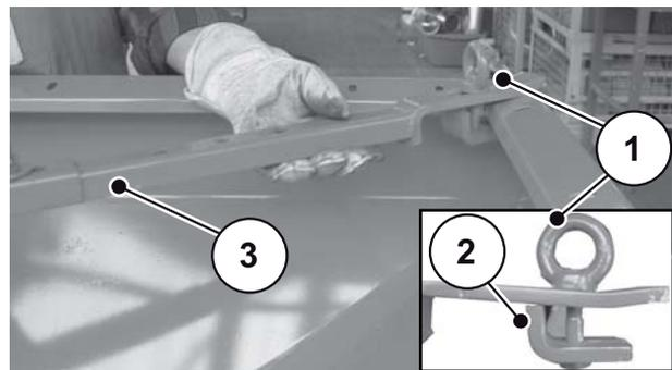
**Figure 5.14:** Fasten the strut to the hopper edge
