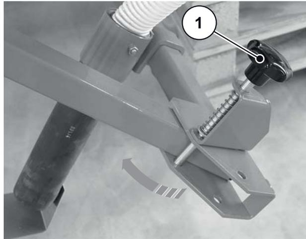
**Figure 7.2:** Fold closed the support frame side part.
