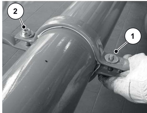
Figure 5.9: Fasten the hose bracket
