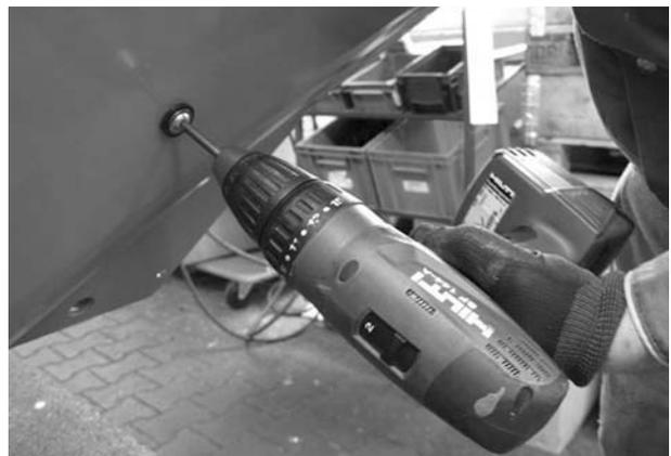
Figure 5.2: Loosen the screws
