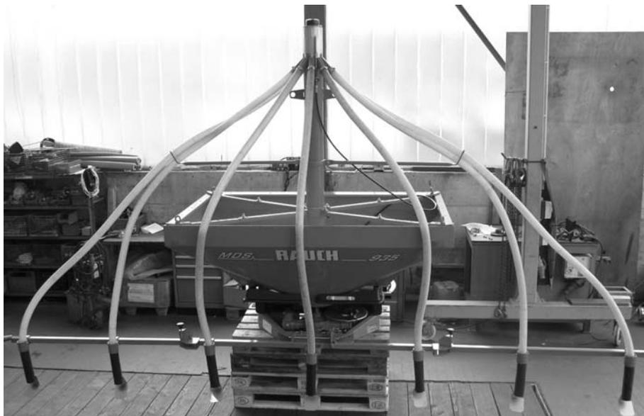
Figure 5.25: Row fertiliser mounted on an MDS fertiliser spreader
