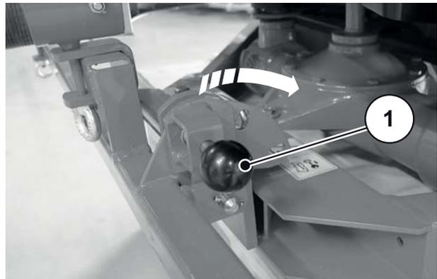
**Figure 7.1:** Swivel the support frame central part
