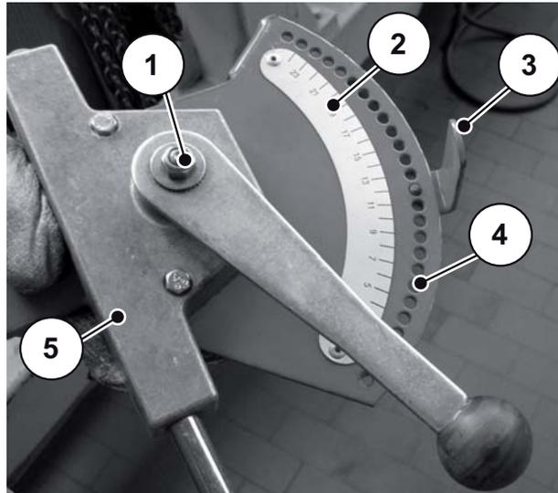
2. Set the stopper lever [3] at the corresponding stop hole of the adjusting segment [4] if required.
