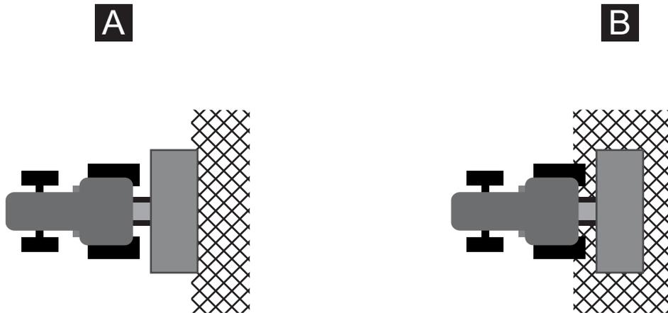
**Figure 3.1:** Hazard zones of row spreading devices
