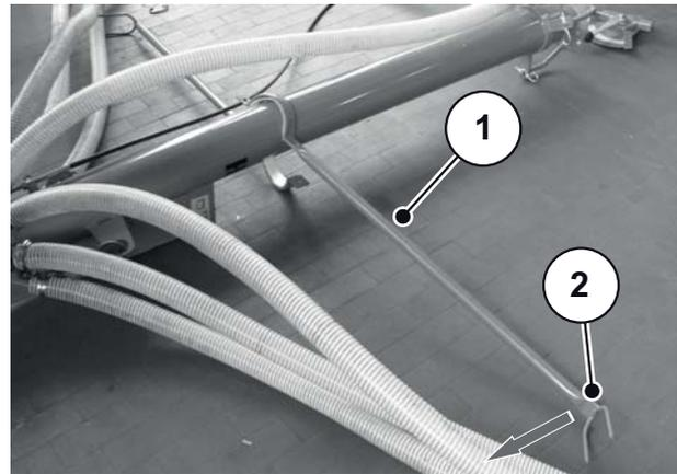
Figure 5.8: Attach hose bracket
