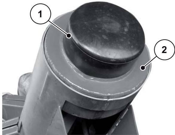
**Figure 9.4:** Remove the pipe plug cap
