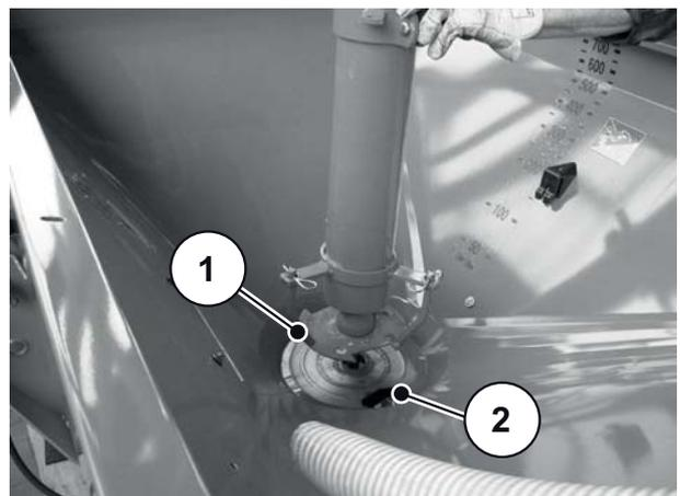
**Figure 5.11:** Lower the assembly into the hopper
