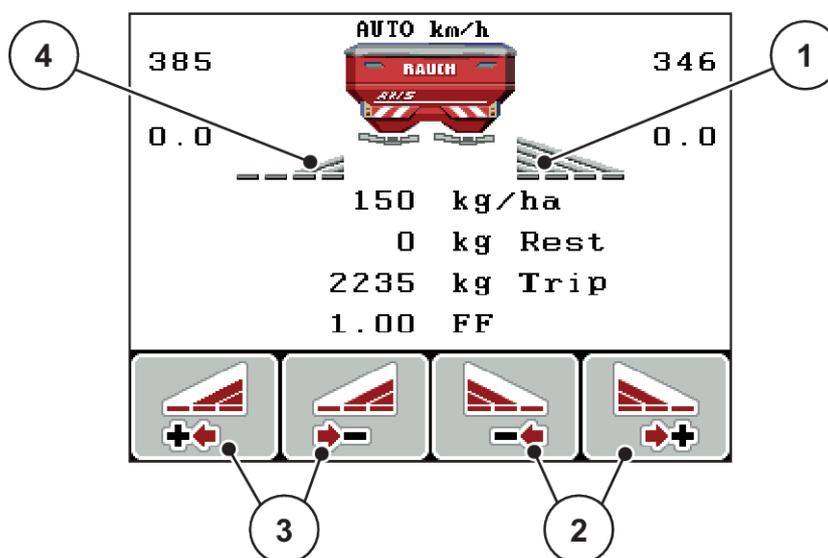
*Fig. 51: Operating screen for spreading operation with sections*
