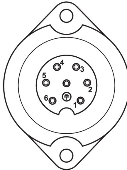
Fig. 10: PIN assignment of the 7-pin plug connector
