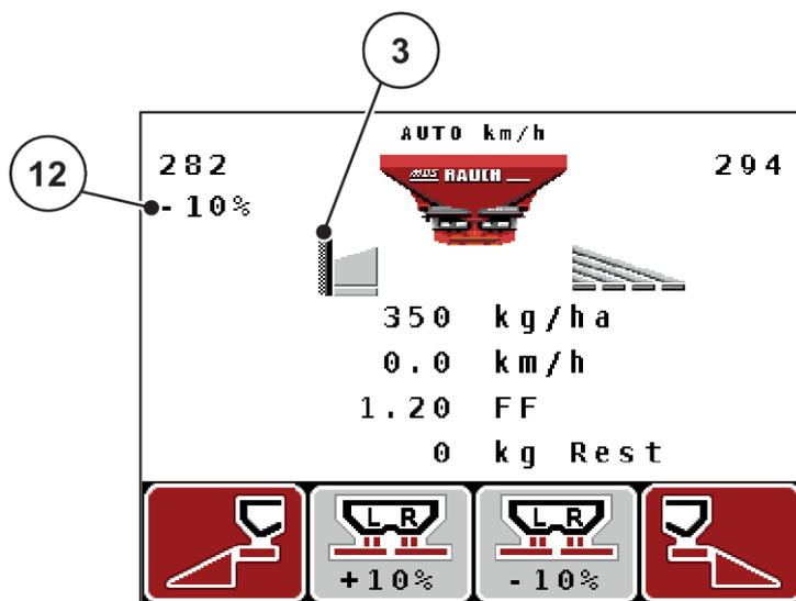
Fig. 5: Control unit display – example MDS operating screen
