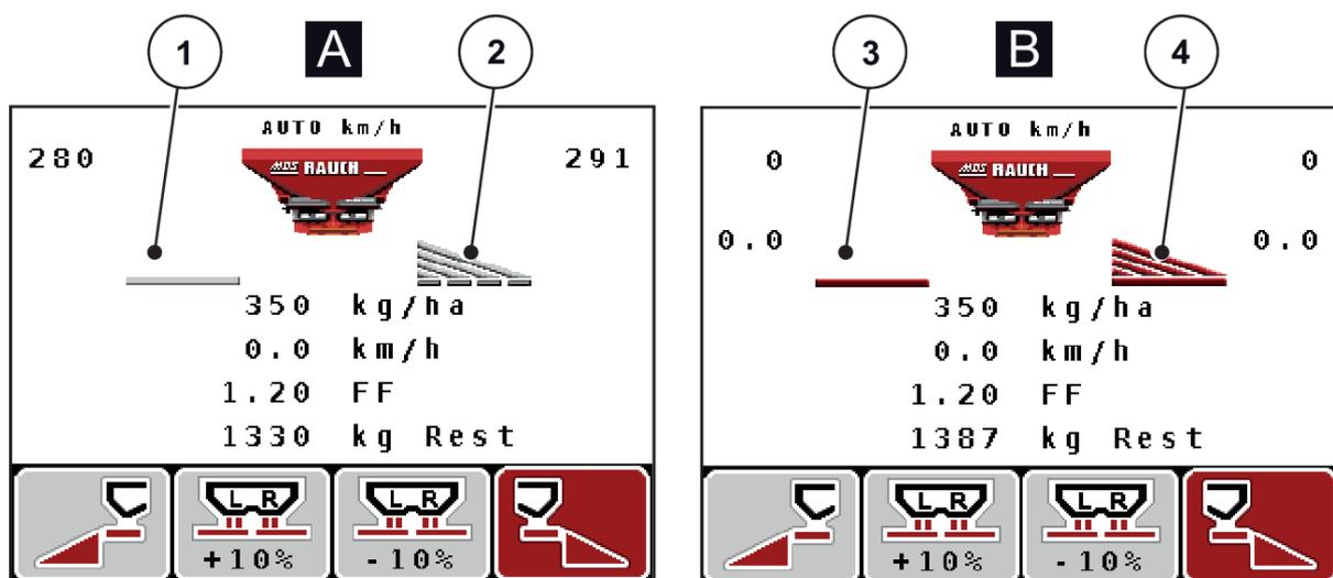
Fig. 7: Display of the MDS metering slide status
