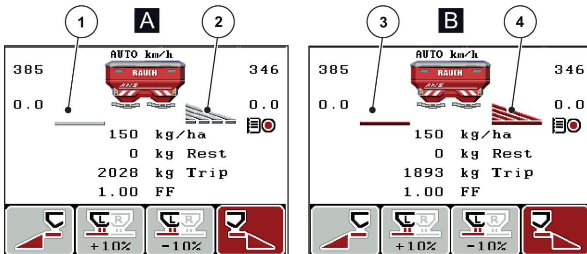
Fig. 6: Display of the AXIS metering slide status
