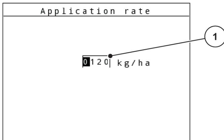
Fig. 49: Input of numerical value (example: application rate)
