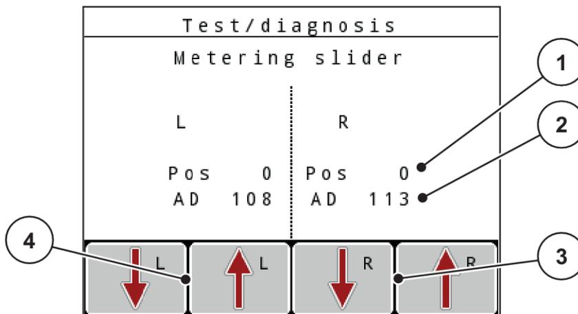
Fig. 43: Test/diagnosis; example: Metering slide
