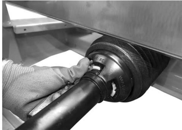
**Figure 7.5:** Secure the universal drive shaft guard
