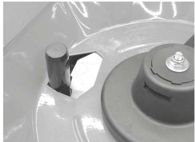
**Figure 12.5:** Lower link pin in metering opening
