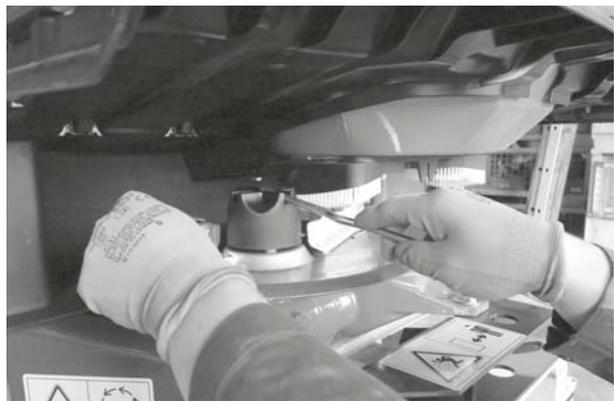
**Figure 12.13:** Loosen cap nut
