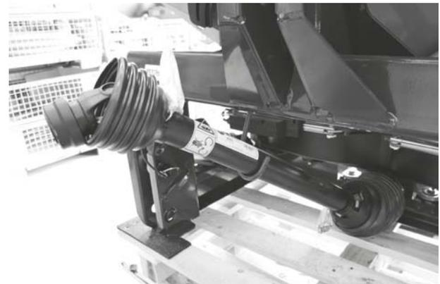
**Figure 7.6:** Retainer of the universal drive shaft
