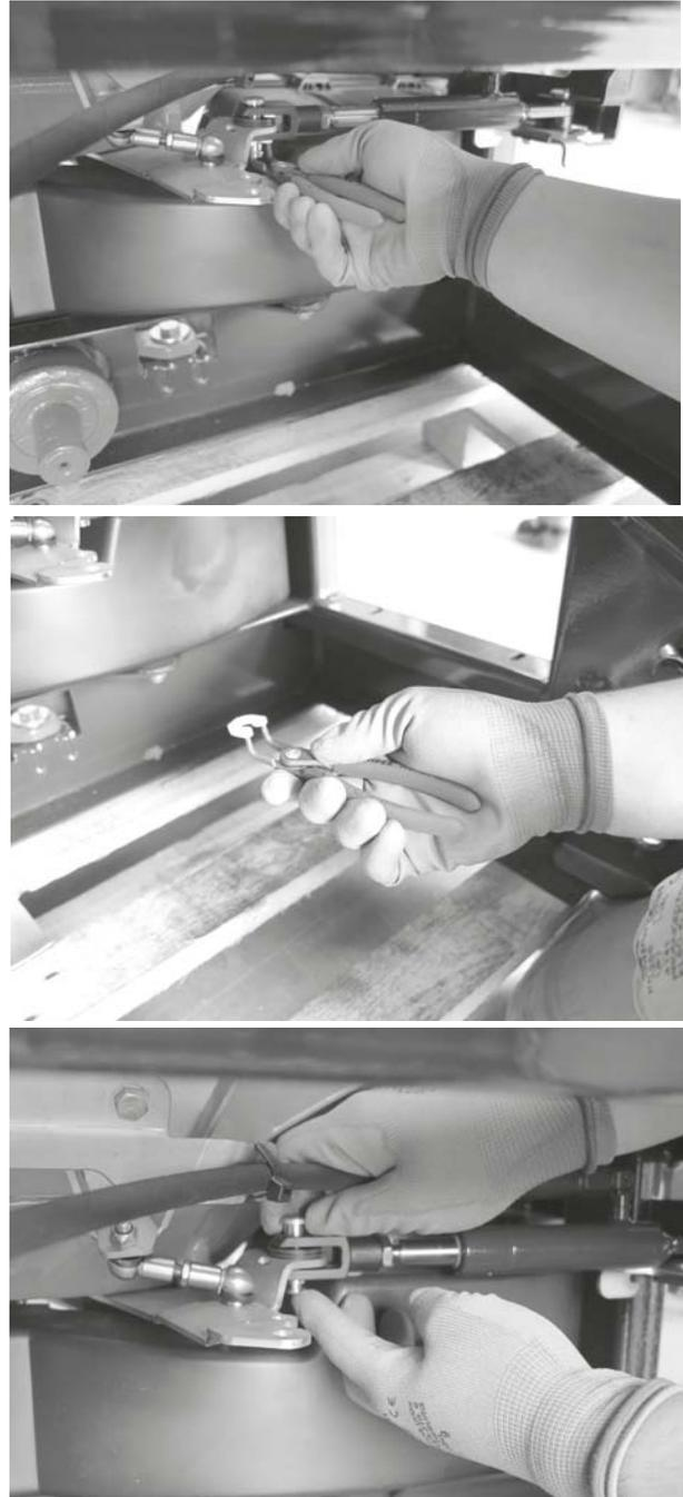
6. Disconnect the metering slide and hydraulic / electric cylinder.
