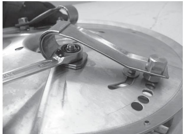
Figure 12.22: Remove the screws
