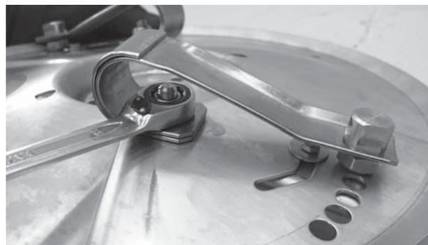
**Figure 12.30:** Fastening the flat springs
