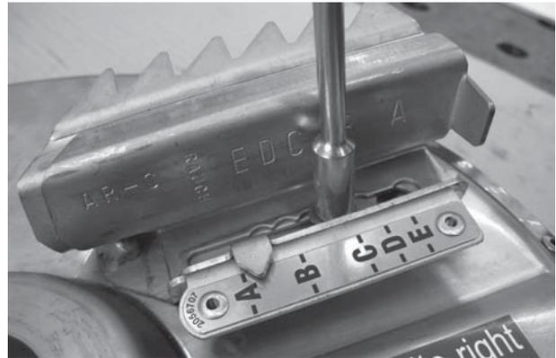
**Figure 12.27:** Spreading vane on the spreading disc
