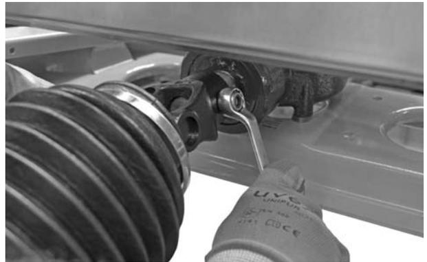
**Figure 7.3:** Connect the universal drive shaft
