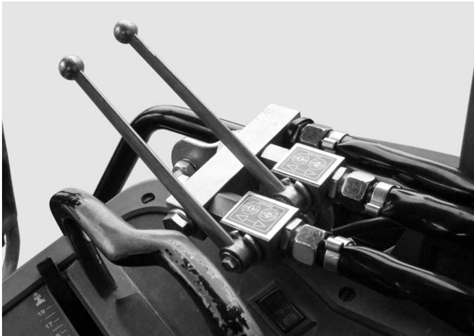
**Figure 7.12:** Metering slide actuator of the two-way unit
