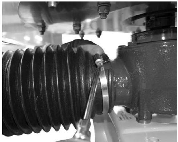
**Figure 7.4:** Mount the universal drive shaft guard
