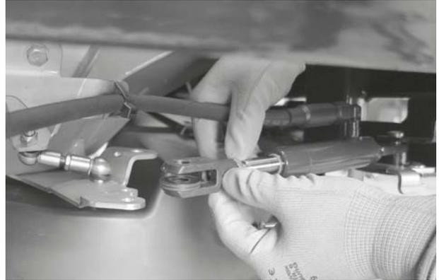
Figure 12.8: Pull out the hydraulic cylinder
