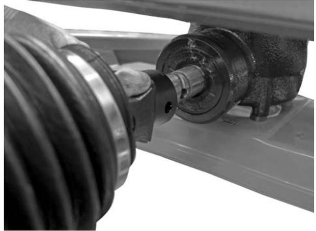
**Figure 7.2:** Push the universal drive shaft onto the transmission spigot
