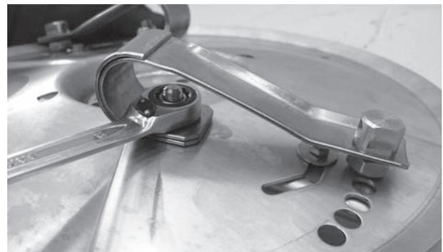
**Figure 9.30:** Fixing the flat spring
