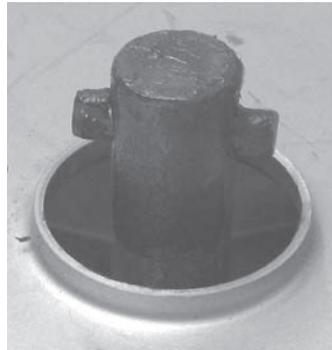
Figure 6.14: Agitator shaft
