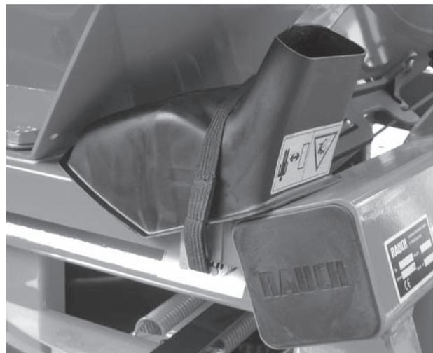
**Figure 8.3:** Calibration test chute
