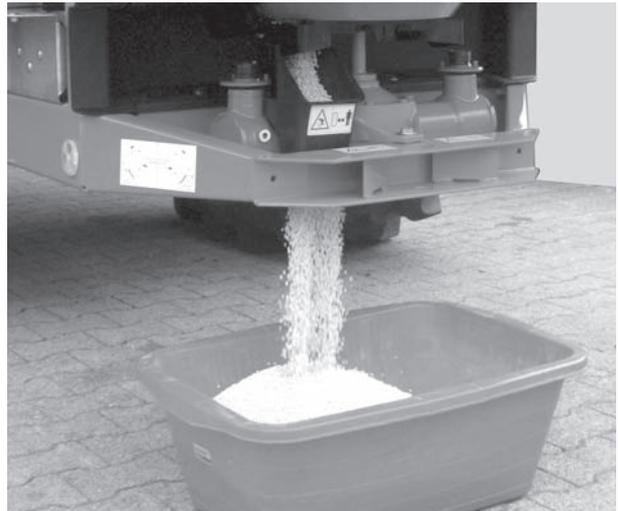
**Figure 8.8:** Running the calibration test
