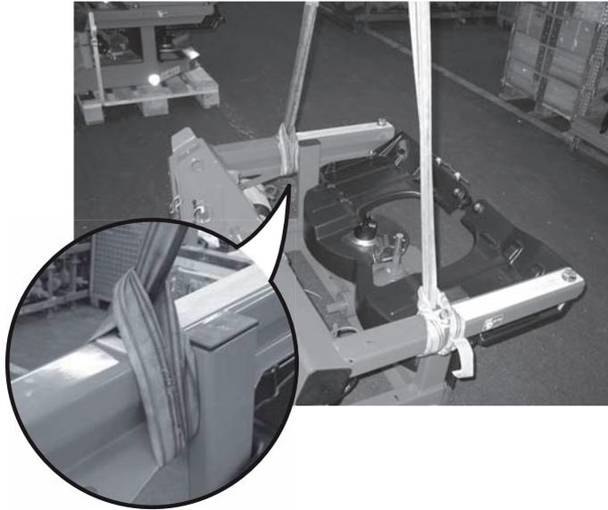
**Figure 6.1:** Lifting the frame
