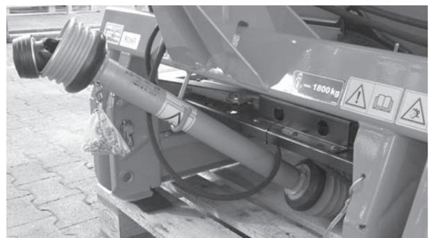
**Figure 6.24:** Universal drive shaft retainer
