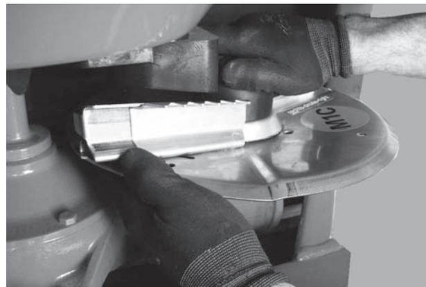
**Figure 8.9:** Screw on cap nuts
