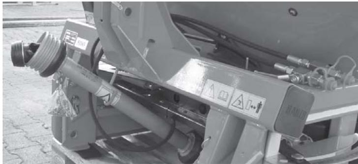
**Figure 5.25:** Parking the universal drive shaft and the hydraulic hoses
