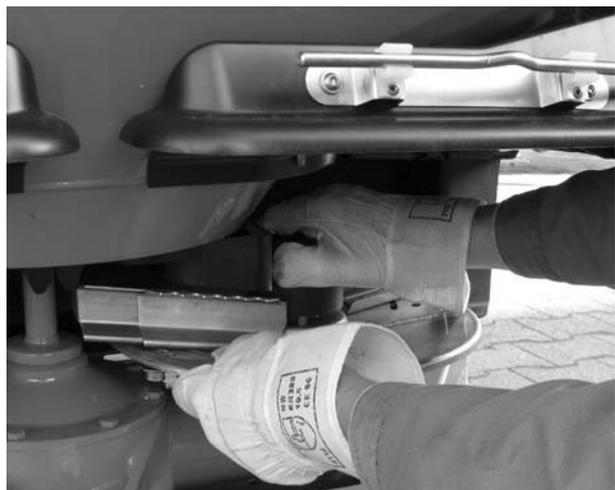
Figure 8.12: Unscrewing cap nuts
