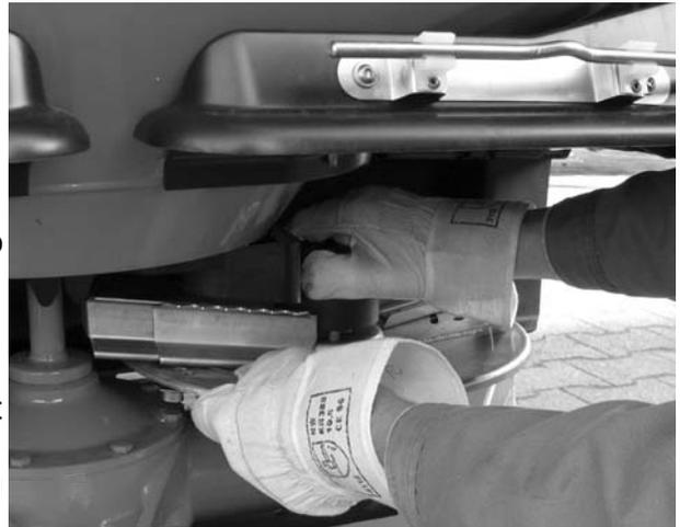
**Figure 7.7:** Screw on cap nuts
