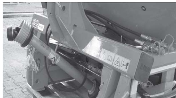
Figure 5.20: Universal drive shaft retainer
