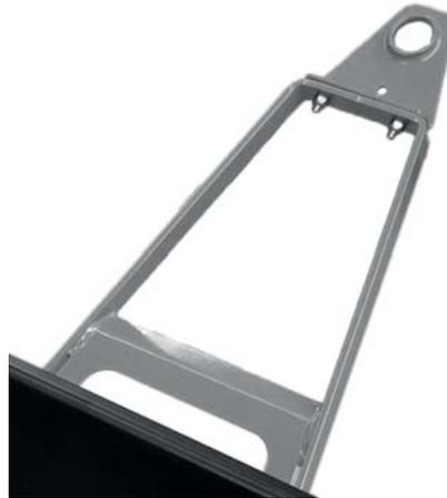
**Figure 6.4:** Towing bar for tractor operation
