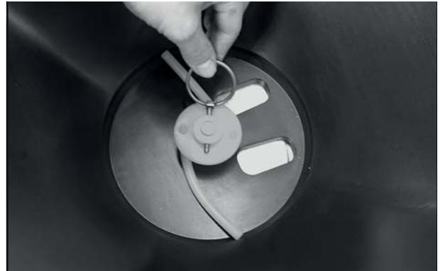
**Figure 9.1:** Agitator in hopper
