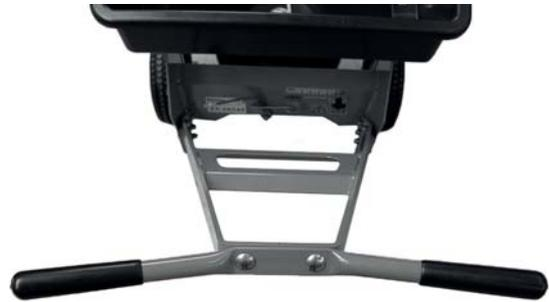
1. Screw the hand grips to the towing bar.
