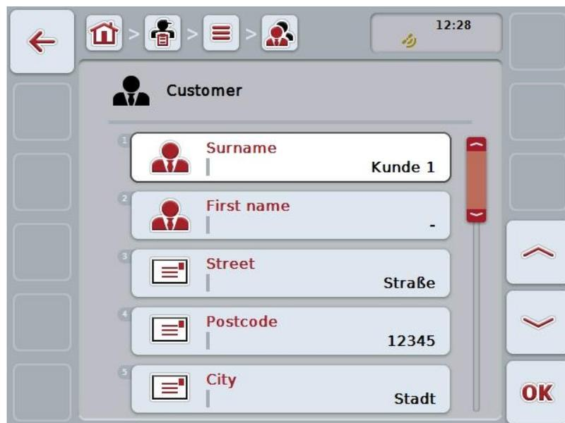
3. In the operating screen, select the parameter for which the value needs to be changed. To do so, press the parameter on the touchscreen or turn the scroll wheel until the button is highlighted in white and then press the scroll wheel.
