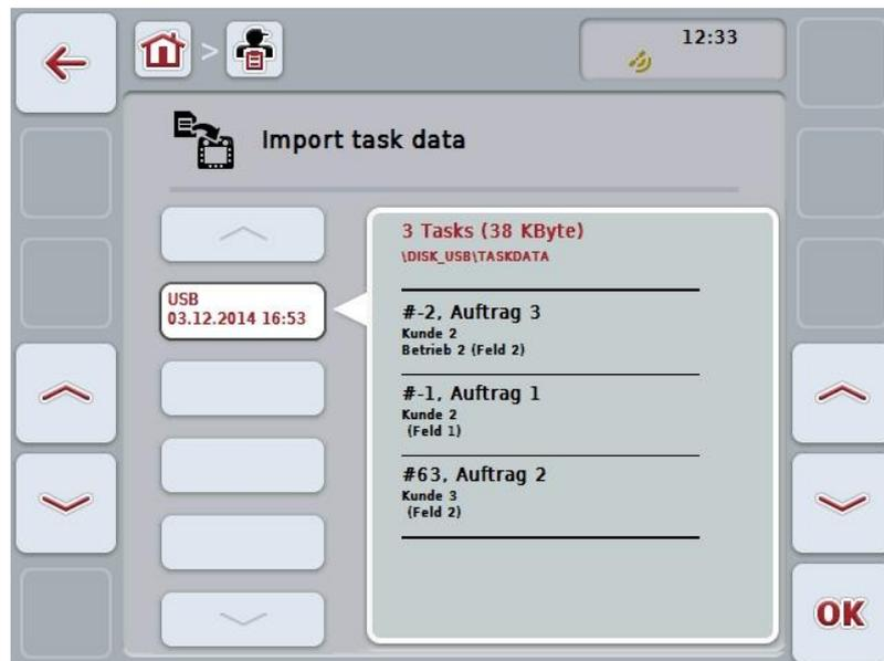
4. Select the task data that needs to be imported. To do so, press the button with the task data on the touchscreen; alternatively, switch between the different sets of task data using the “Up” (F10) and “Down” (F11) buttons or turn the scroll wheel until the required button is highlighted in white and press the “OK” button (F6).
