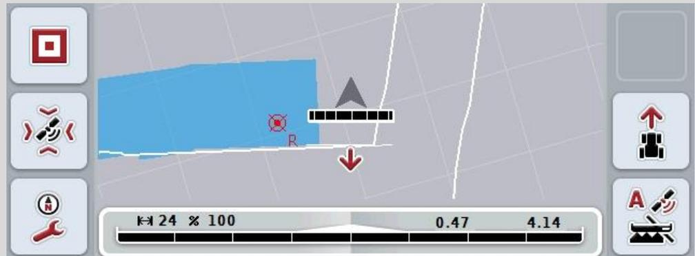
If the indicated driving direction does not correspond to the actual driving direction, you can correct the driving direction manually (see chapter 4.4.9).
