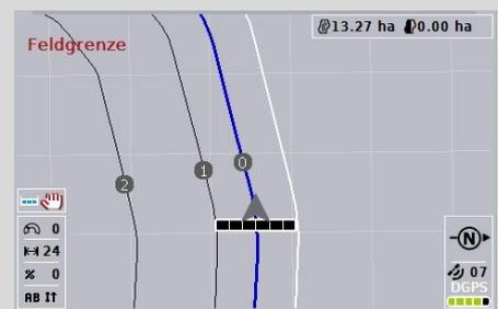
Lead tracks are displayed in the headland. The reference for these lead tracks is the field boundary.
