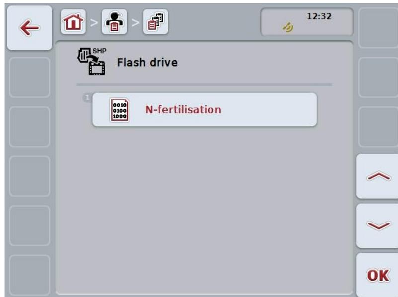
5. Select the application map that is to be imported. To do so, press the button with the required application map on the touchscreen or turn the scroll wheel until this button is highlighted in white and then press the "OK" button (F6).
