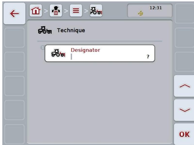
2. In the operating screen, select all parameters one after the other. To do so, press the parameter on the touchscreen or turn the scroll wheel until the button is highlighted in white and then press the scroll wheel. Once the parameter is highlighted you can, alternatively, also press the "OK" (F6) button.
