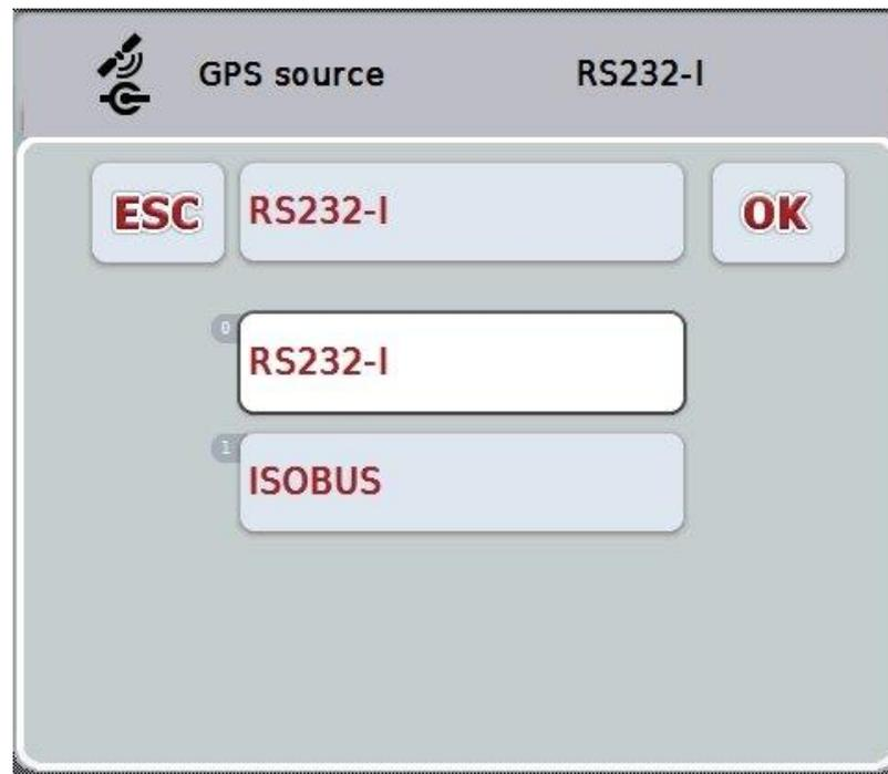
2. Select the desired GPS source in the selection list. To do so, on the touchscreen press on the button with the GPS source or turn the scroll wheel until the button is highlighted in white. The GPS source then appears in the selection window.
