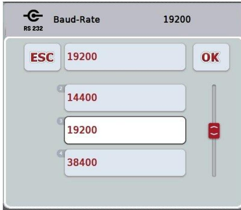
3. Select the desired baud-rate in the selection list. To do so, on the touchscreen press on the button with the baud-rate or turn the scroll wheel until the button is highlighted in white. The baud-rate then appears in the selection window.
