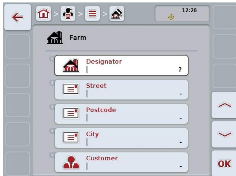
2. In the operating screen, select all parameters one after the other. To do so, press the parameter on the touchscreen or turn the scroll wheel until the button is highlighted in white and then press the scroll wheel. Once the button is highlighted you can, alternatively, also press the "OK" (F6) button.
