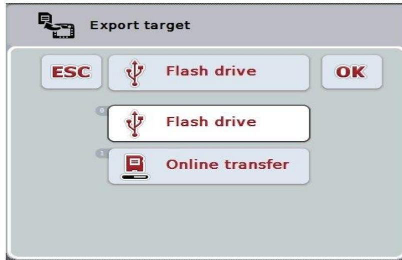
2. Select either “Flash drive” or “Online transfer”. To do so, press the button on the touchscreen with the required transfer path or turn the scroll wheel until this button is highlighted in white and then press the scroll wheel. Once the button is highlighted you can, alternatively, also press the "OK" button.
