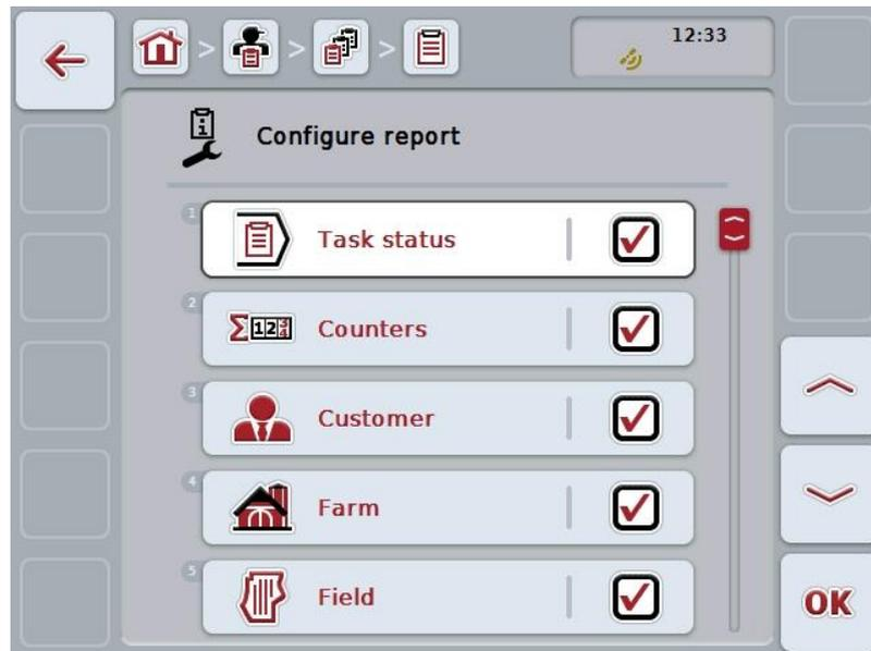
2. Select the parameters which need to be displayed in the task report. To do so, press the parameter on the touchscreen or turn the scroll wheel until the button is highlighted in white and then press the scroll wheel. Once the button is highlighted you can, alternatively, also press the "OK" (F6) button.
