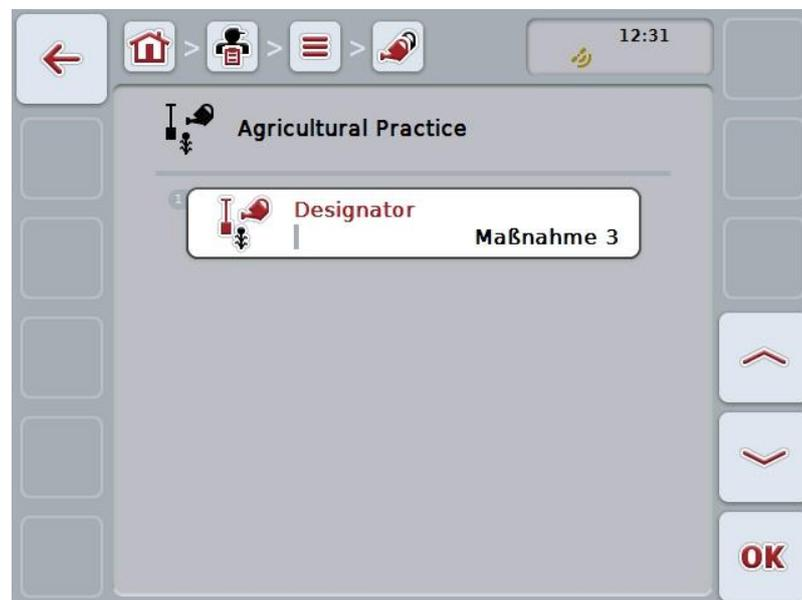
3. In the operating screen, select the parameter for which the value needs to be changed. To do so, press the parameter on the touchscreen or turn the scroll wheel until the button is highlighted in white and then press the scroll wheel. Once the button is highlighted you can, alternatively, also press the "OK" (F6) button.
