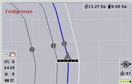
*Guidance tracks* are displayed in the headland. The reference for these *guidance tracks* is the field boundary. The headland can be worked.
