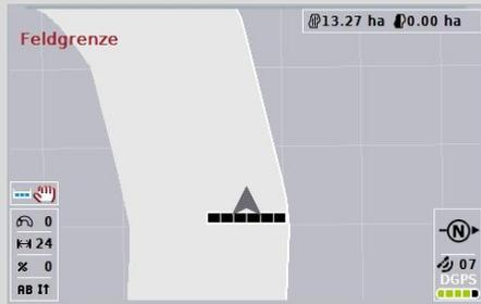
The headland is plotted in light grey, the sections are automatically switched off in this area. The inner field can be worked.
