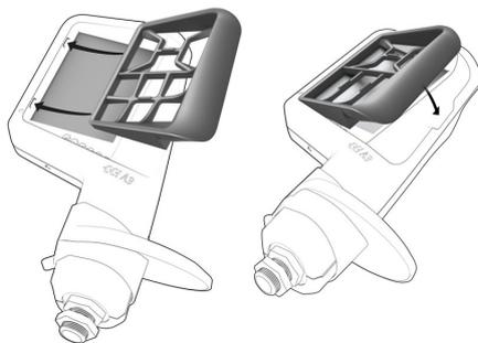
1. Insert the two pegs on the grid into the grooves in the casing of the CCI A3.
