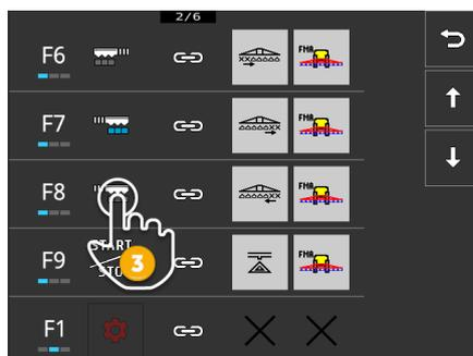
3. Navigate to the operating element using the "Down" / "Up" buttons and press the button with the pictogram that is to be changed.
