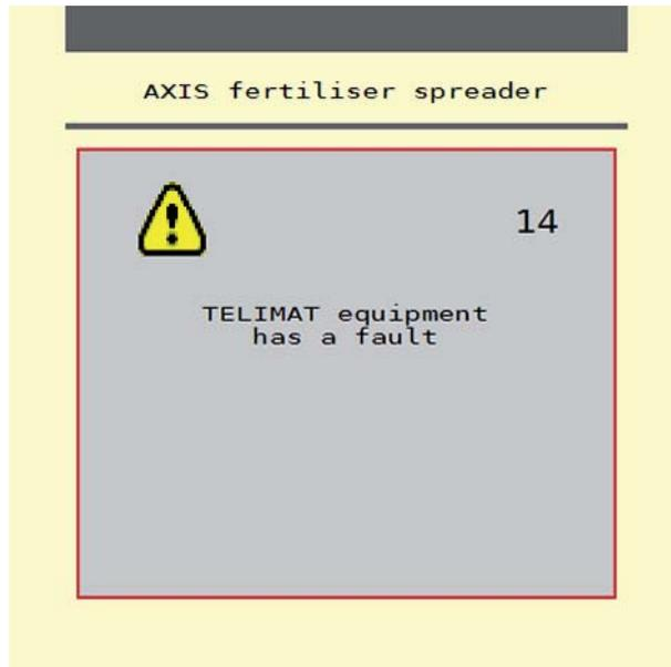
**Figure 5.2:** TELIMAT alarm message display
