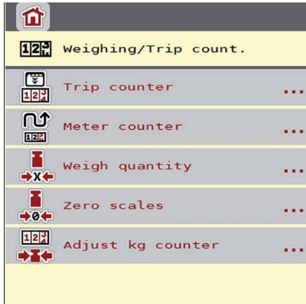
Figure 4.18: Weighing trip counter menu
