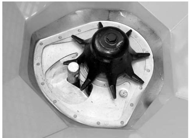
1. Insert a lower link pin with a diameter of **28 mm** centrally into the metering opening.
