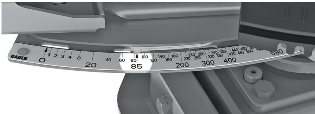
**Figure 9.16:** Metering slide pointer on position 85
