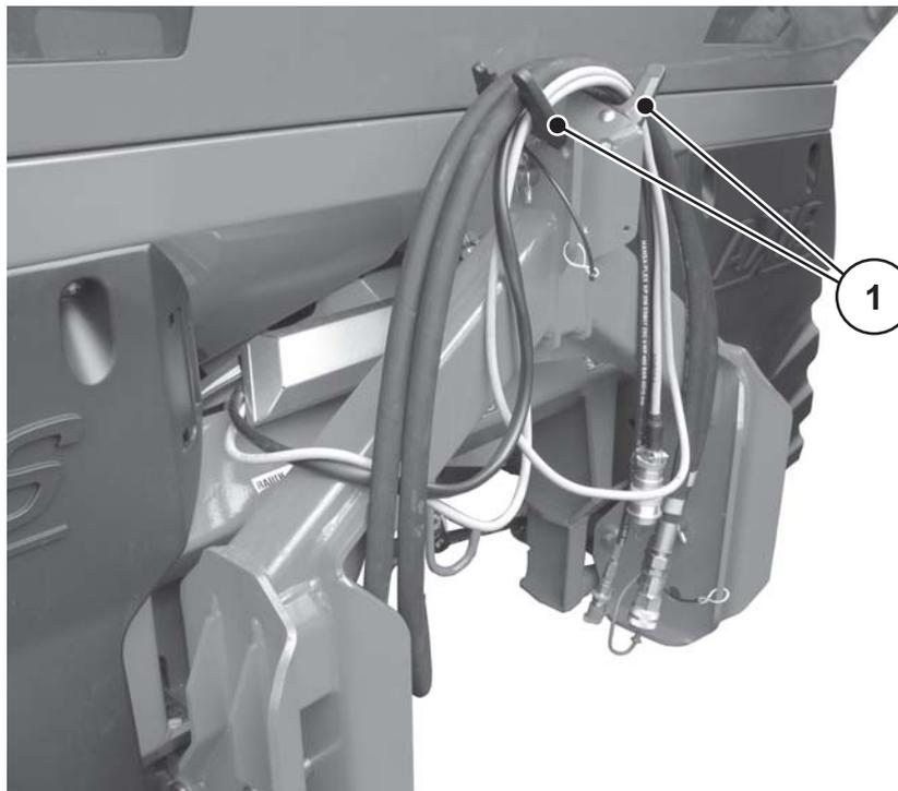
**Figure 8.9:** Storage of cables and hydraulic hoses
