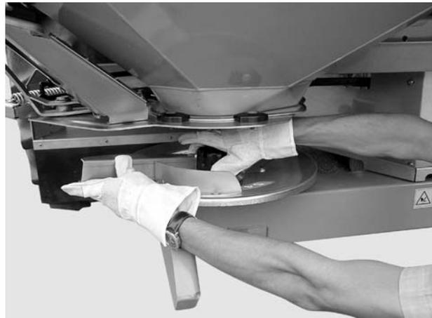
**Figure 8.4:** Unscrew the cap nut
