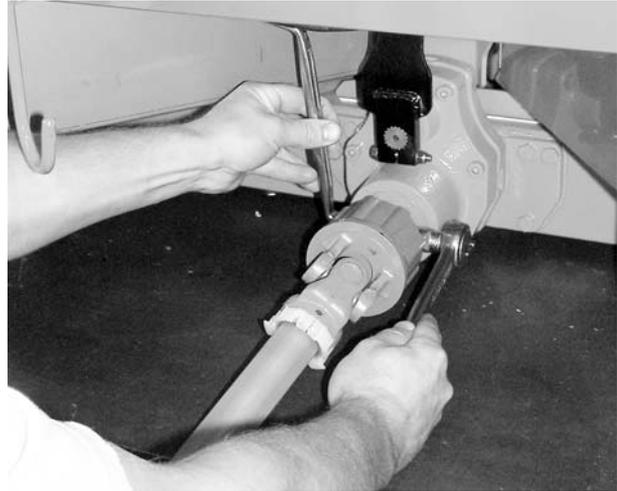
**Figure 8.3:** Tighten the universal drive shaft
