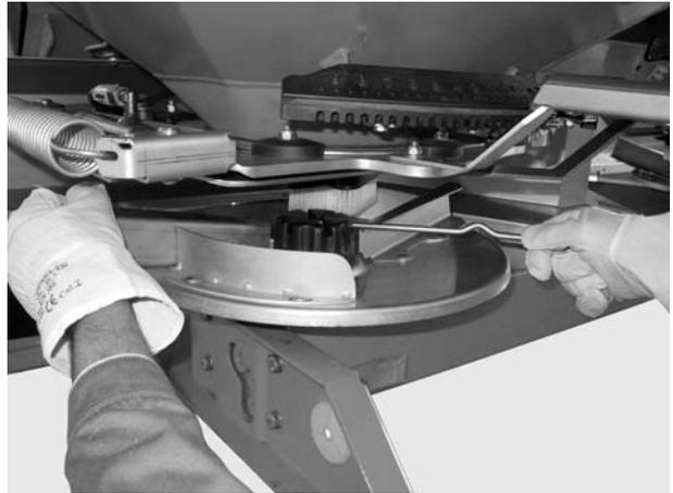
**Figure 11:** Loosen the cap nut
