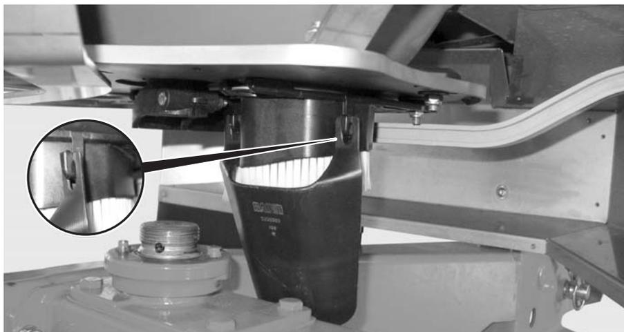
**Figure 12:** Attach the calibration test chute
