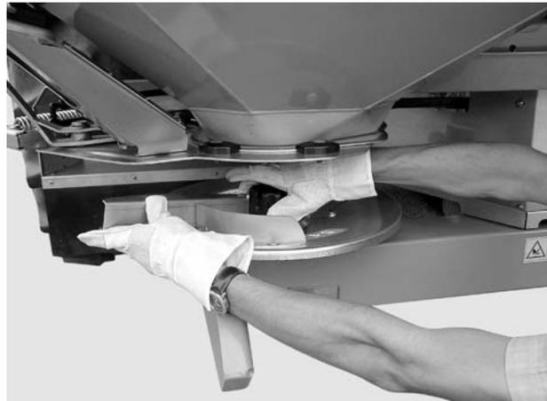
**Figure 13:** Screw on the cap nut
