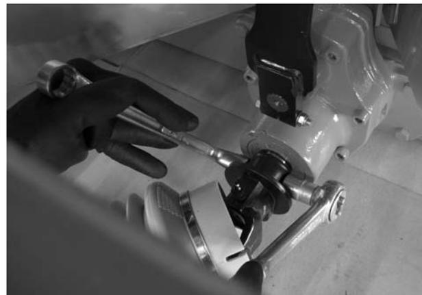
Figure 4: Tighten the universal drive shaft
