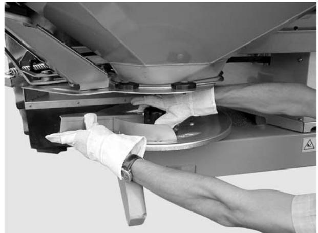
**Figure 12:** Unscrew the cap nut
