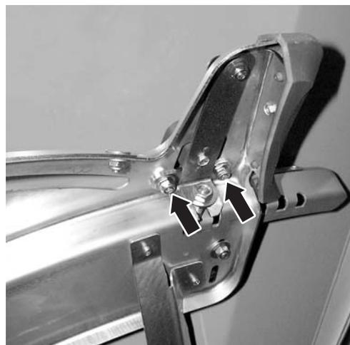
**Figure 29:** Loosen the drop point adjustment plate
