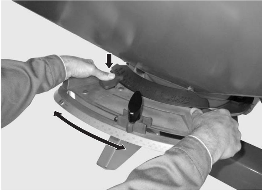
**Figure 13:** Adjustment centre for drop point
