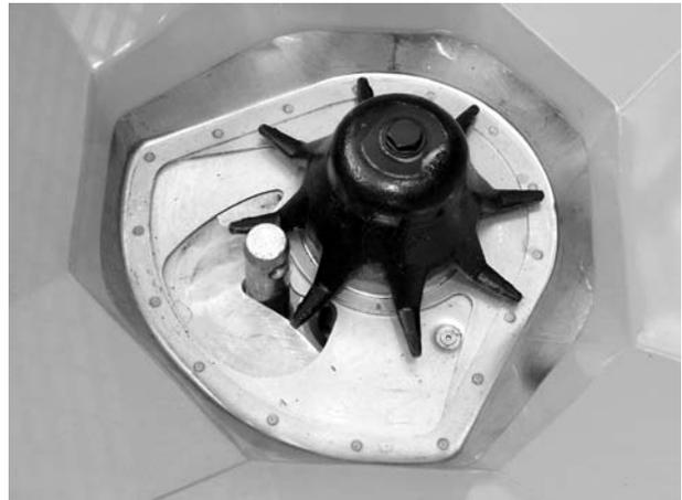
**Figure 23:** Lower link pin in metering opening
