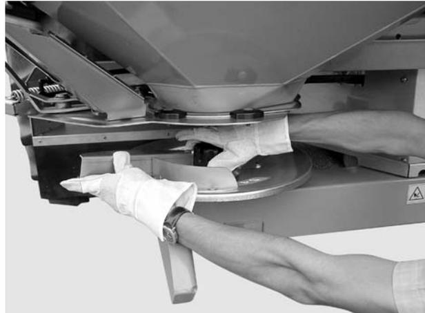
Figure 5: Unscrew the cap nut
