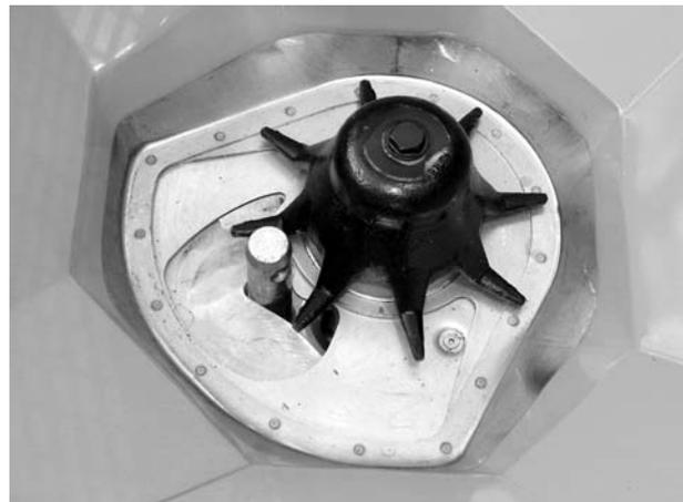
**Figure 22:** Lower link pin in metering opening
