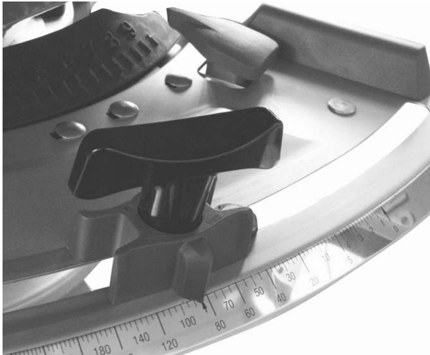
**Figure 26:** Adjustment scale of metering slide
