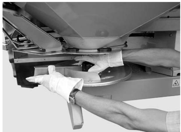
**Figure 20:** Screw on the cap nut
