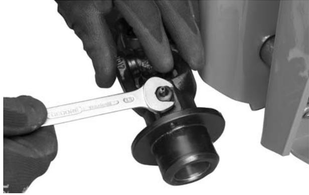
Figure 2: Remove lubricating nipples
