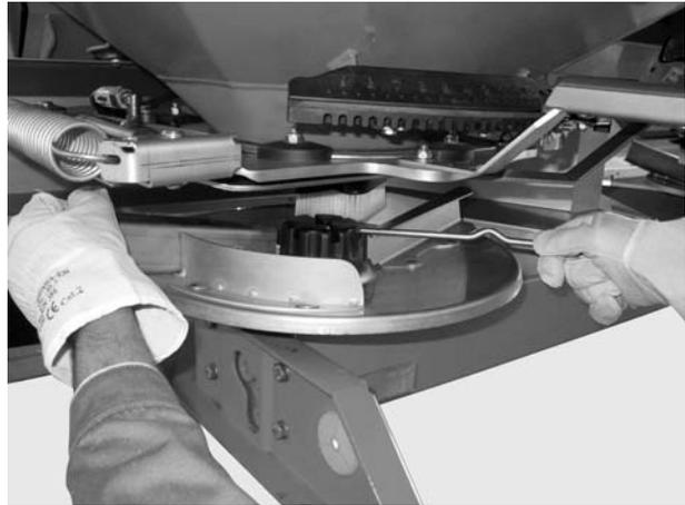
**Figure 17:** Loosen the cap nut
