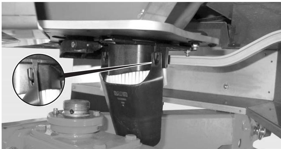
**Figure 18:** Attach the calibration test chute
