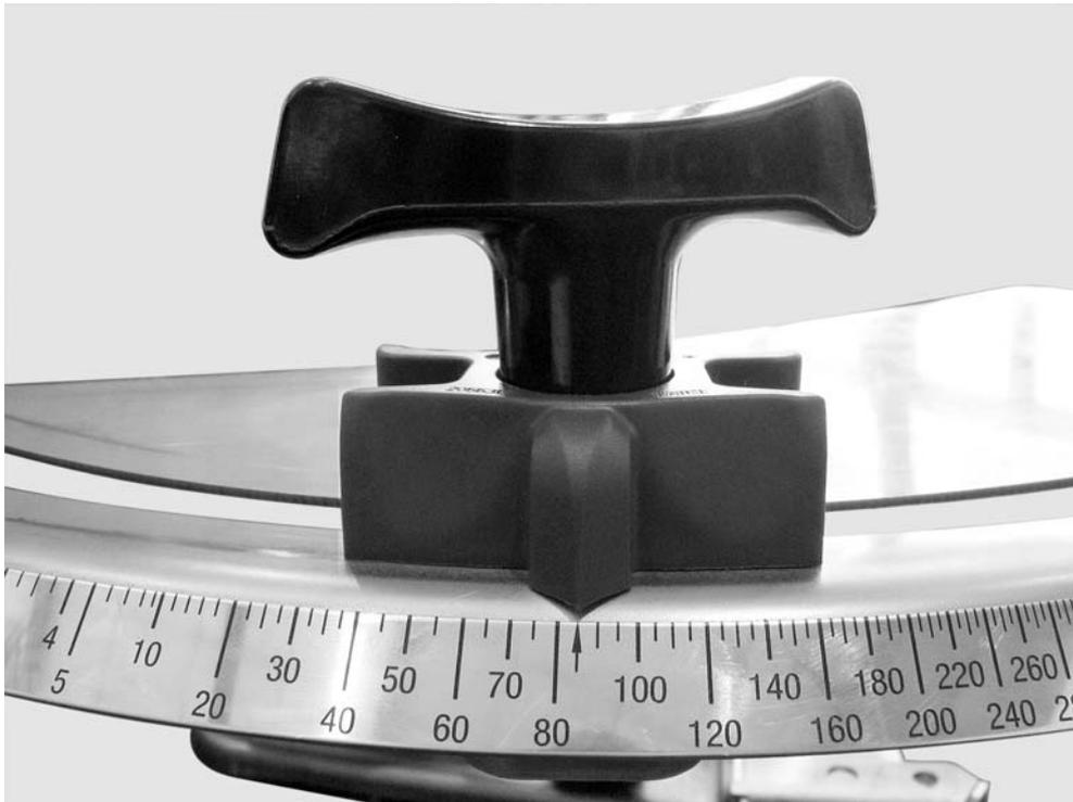
**Figure 24:** Adjustment scale of metering slide
