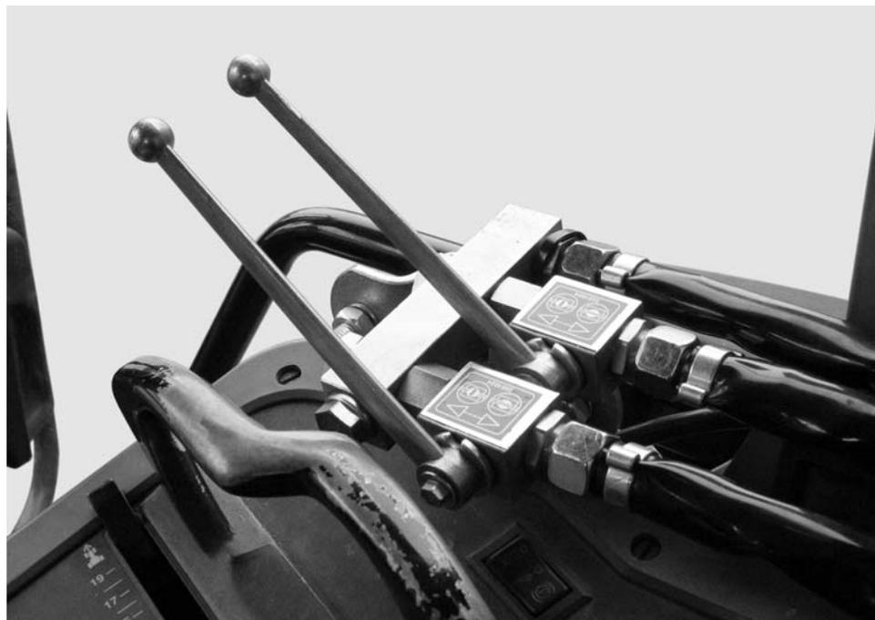
**Figure 8:** Slide actuator of the two-way unit
