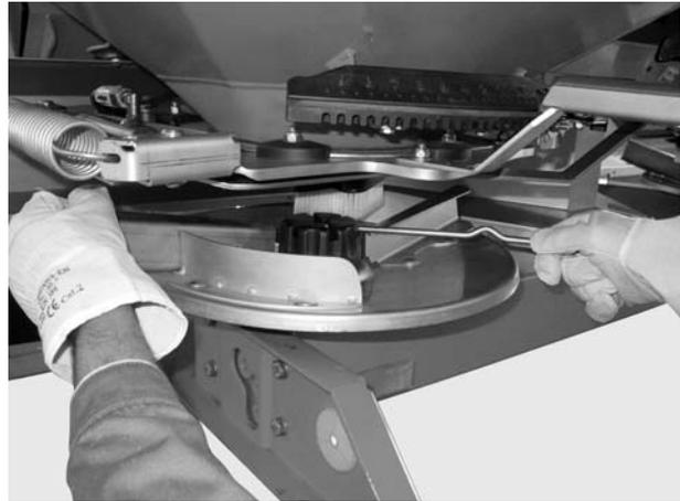
**Figure 10:** Loosen the cap nut
