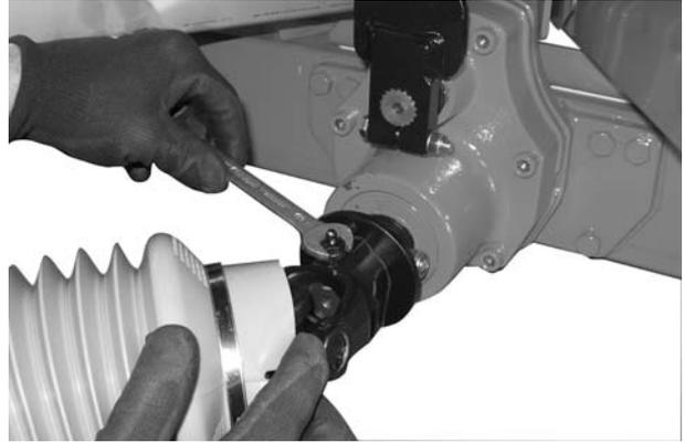
**Figure 5:** Tighten lubricating nipples
