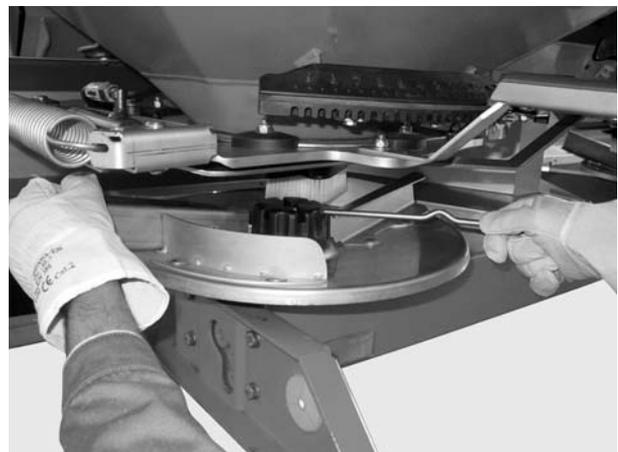
1. Remove the adjustment lever from the bracket.
