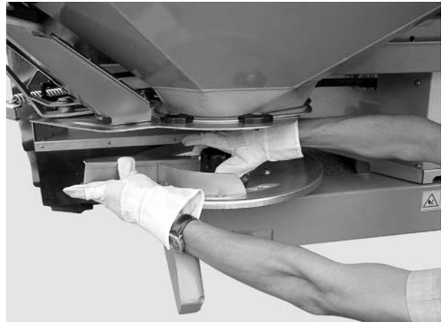
**Figure 14:** Screw on the cap nut
