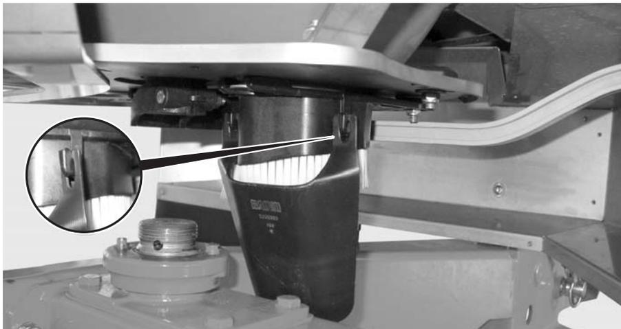
**Figure 11:** Attach the calibration test chute
