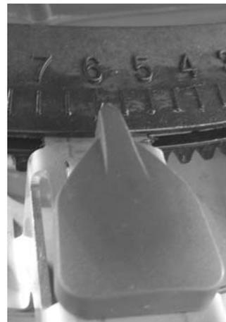
**Figure 27:** Setting the drop point to position 6.
