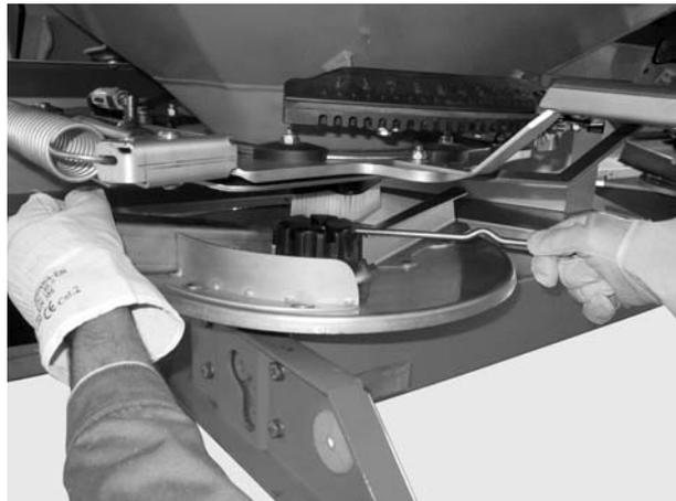
**Figure 8.3:** Release cap nuts
