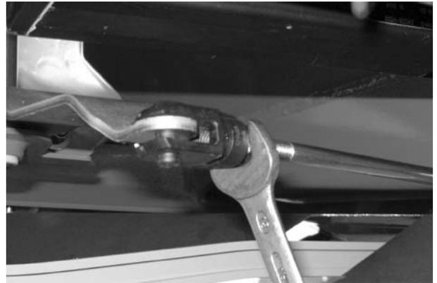
**Figure 9.19:** Engaging the inner yoke
