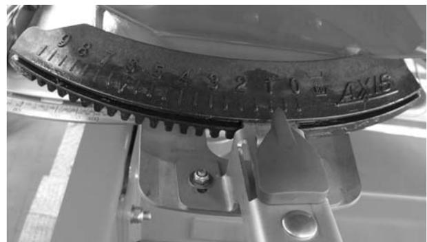
**Figure 9.30:** Checking the adjustment of the drop point
