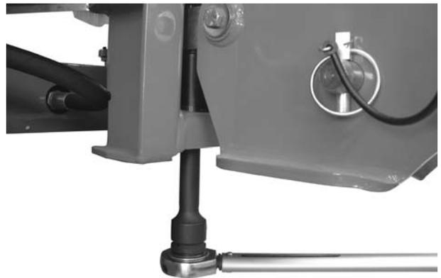
**Figure 9.1:** Fasten the weighing cell (on the left of the travelling direction)
