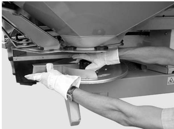
**Figure 8.4:** Unscrewing cap nuts
