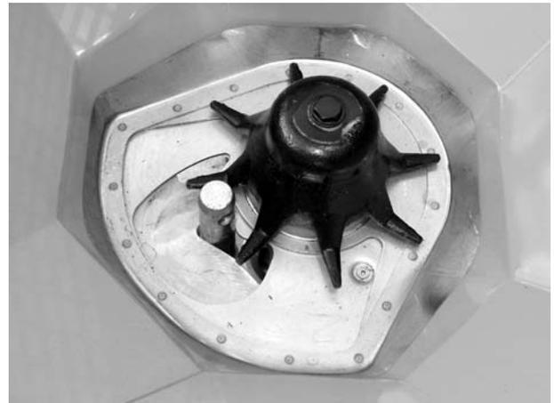
**Figure 9.13:** Lower link pin in metering outlet
