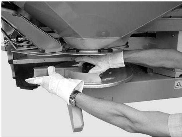
**Figure 21:** Screw on the cap nut
