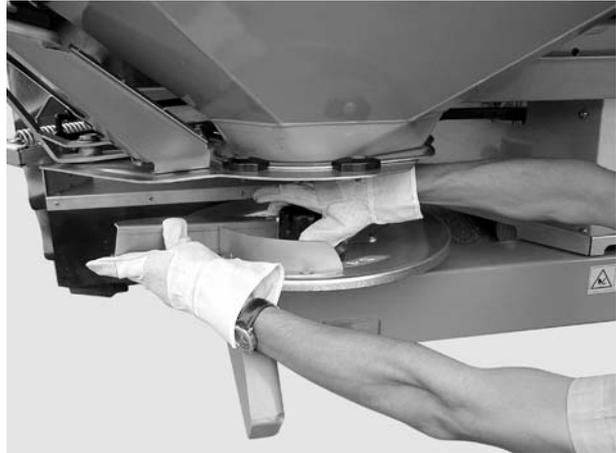
**Figure 5:** Unscrew the cap nut
