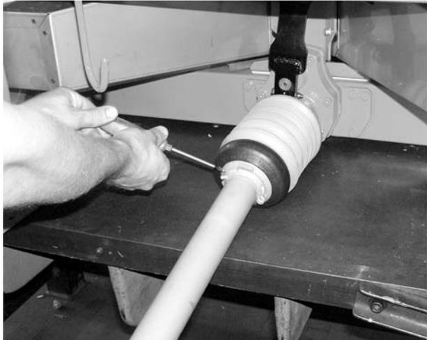
**Figure 8.5:** Secure universal drive shaft guard
