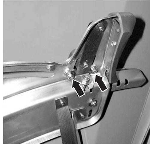
**Figure 34:** Loosen the drop point adjustment plate
