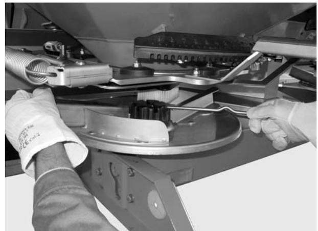
1. Use the adjustment lever to loosen the cap nut of the spreading disc. Remove the spreading discs from the hub.
