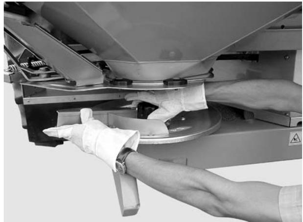
**Figure 14:** Screwing on the cap nuts
