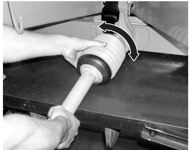
**Figure 6:** Put the universal drive shaft guard back on
