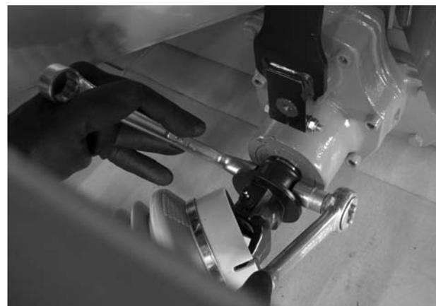
Figure 4: Tighten drive shaft
