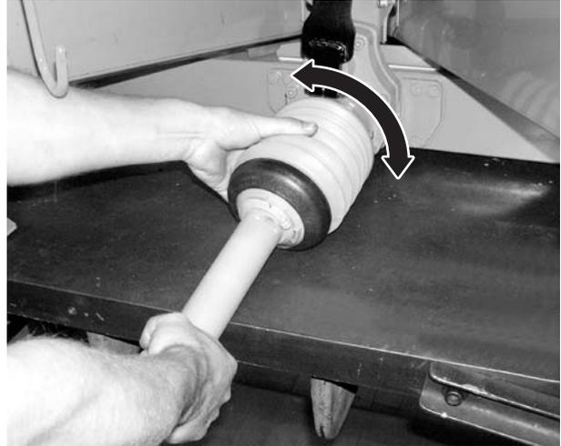
**Figure 8.4:** Put the universal drive shaft guard back on
