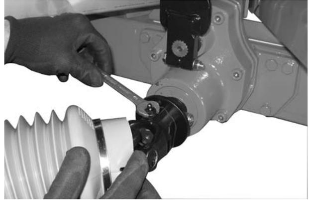
**Figure 5:** Tighten lubricating nipples
