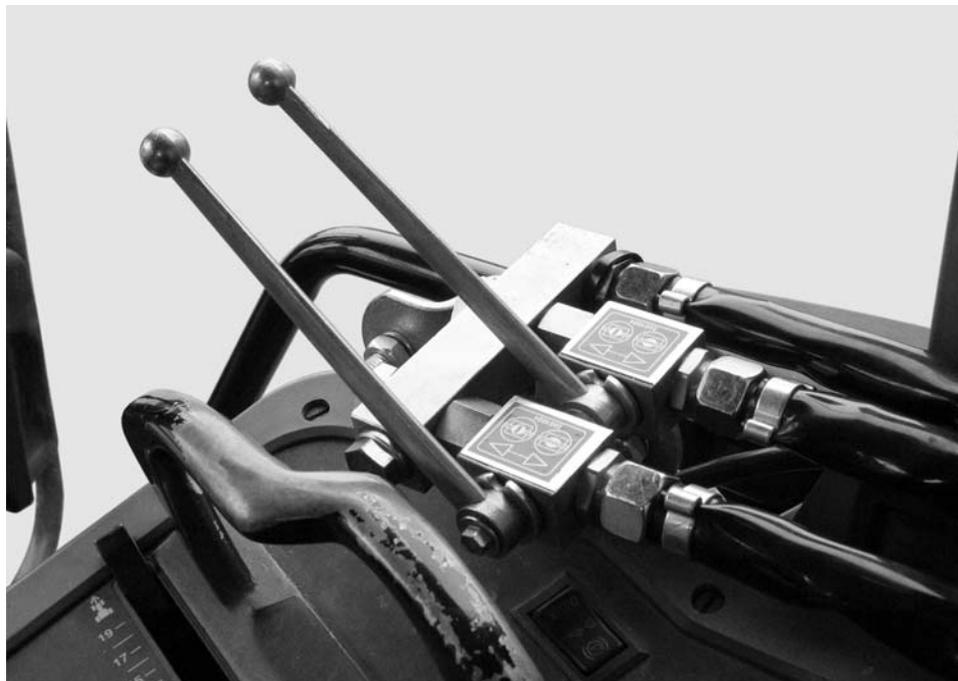
**Figure 1:** Slide actuator of the two-way unit
