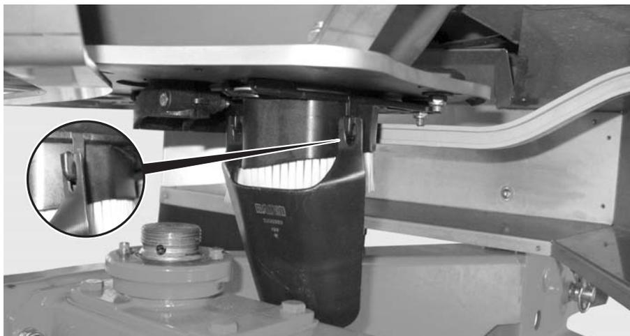
**Figure 19:** Attaching the calibration test chute
