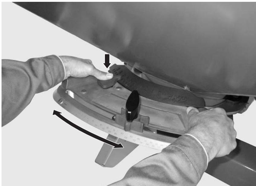
**Figure 14:** Adjustment centre for drop point
