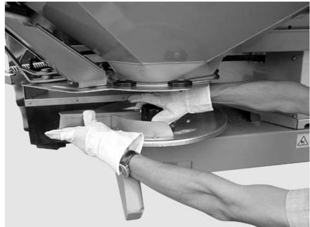
**Figure 6:** Unscrew the cap nut
