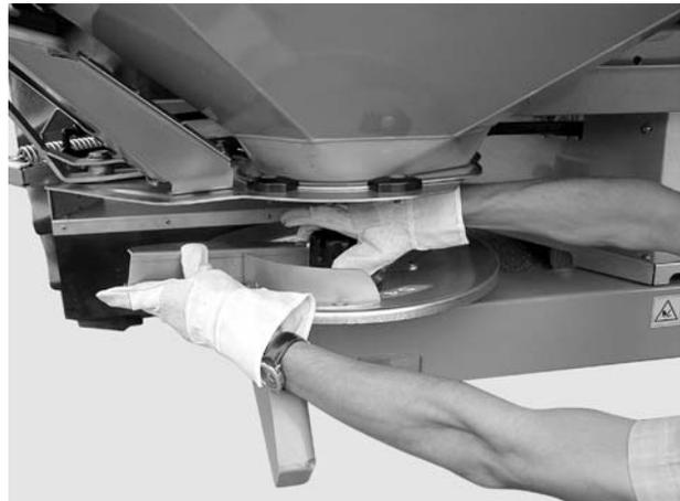
**Figure 14:** Screwing on the cap nuts
