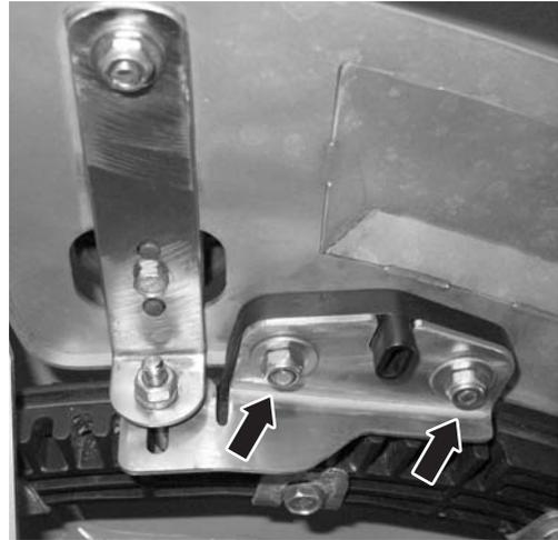
**Figure 28:** Loosen the drop point adjustment plate
