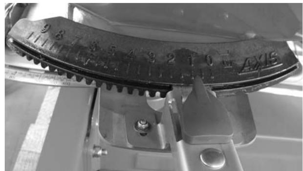
**Figure 42:** Checking the adjustment of the drop point
