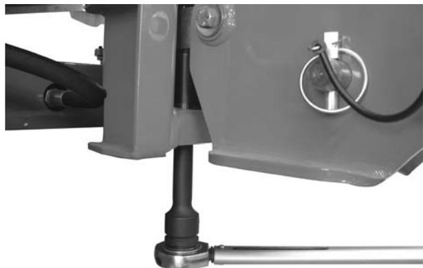
**Figure 18:** Fastening the weighing cell (on the left side of the direction of travel)
