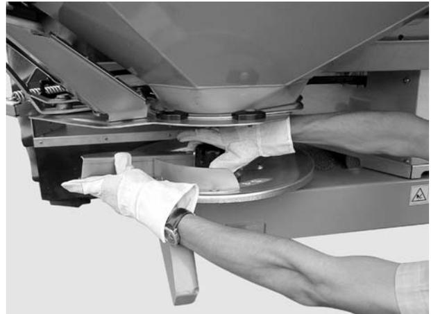
**Figure 13:** Unscrew the cap nut
