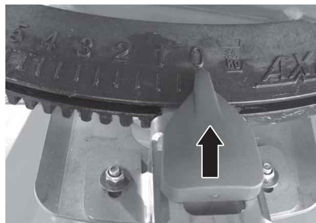
Bild 39: Set the drop point to position 0.
