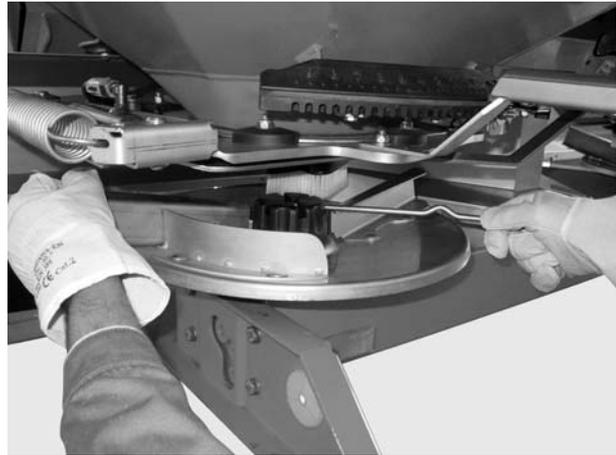
**Figure 18:** Loosen cap nut
