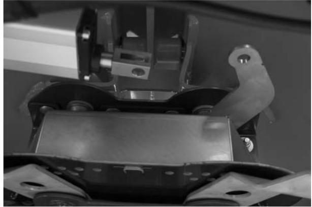
Figure 27: Disengaging the actuator
