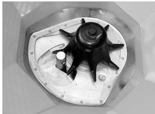
Figure 20: Lower link pin in metering opening
