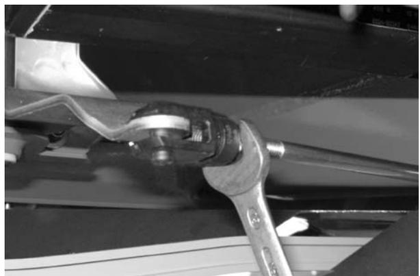
Figure 29: Engaging the inner yoke
