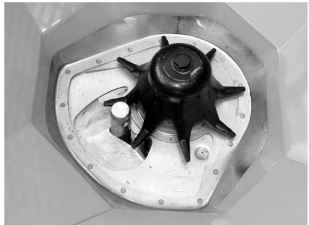
**Figure 25:** Lower link pin in metering opening
