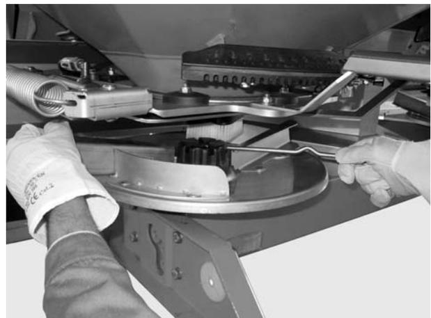
**Figure 11:** Loosen cap nut
