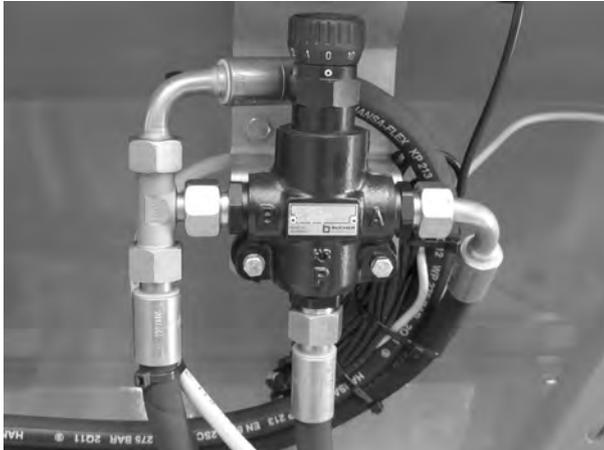
Fig. 22: Flow control valve
