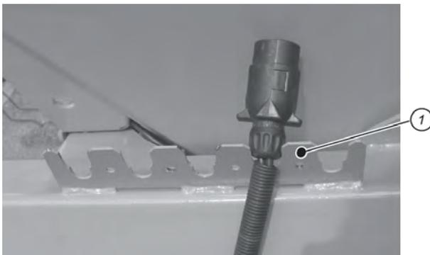
*Fig. 36: Bracket for cables and hoses*
