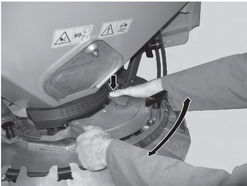
Fig. 28: Drop point adjustment center
