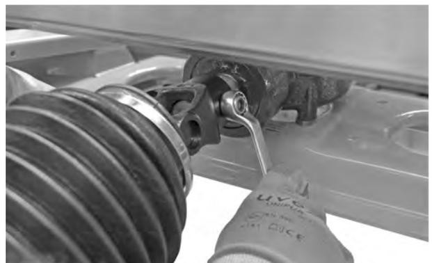
*Fig. 17: Connecting the universal drive shaft*
