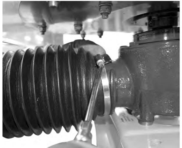
*Fig. 18: Mounting the universal drive shaft guard*
