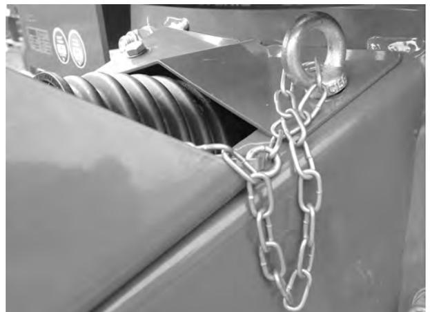
*Fig. 22: Securing the safety chain*
