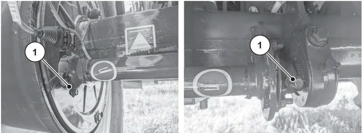
Fig. 61: Rigid axle brake camshaft bearing
