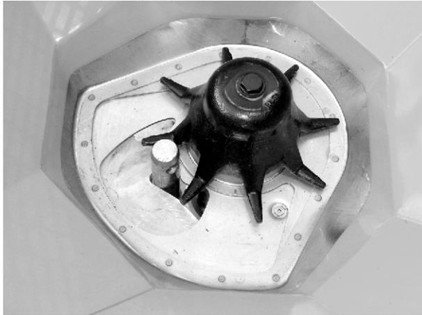
*Fig. 87: Lower link pin in metering opening*
