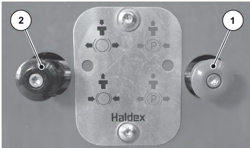
Fig. 78: Pneumatic brake
