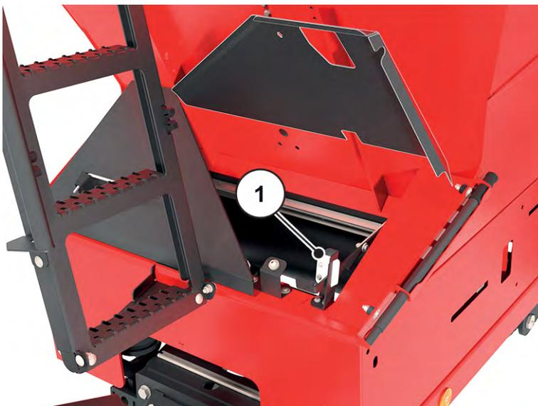
Fig. 32: Cleaning flap in closed position, front in direction of travel
