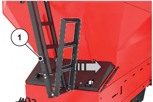
Fig. 33: Folding out the lower part of the ladder
