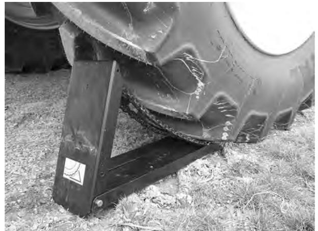
*Fig. 48: Positioning the wheel chock*
