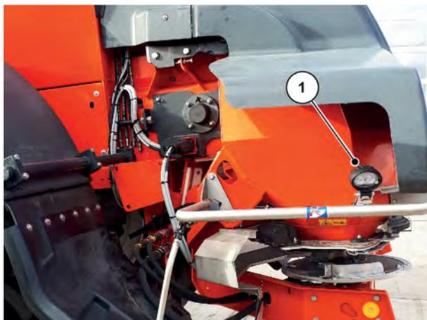
Fig. 17: SpreadLight optional equipment
