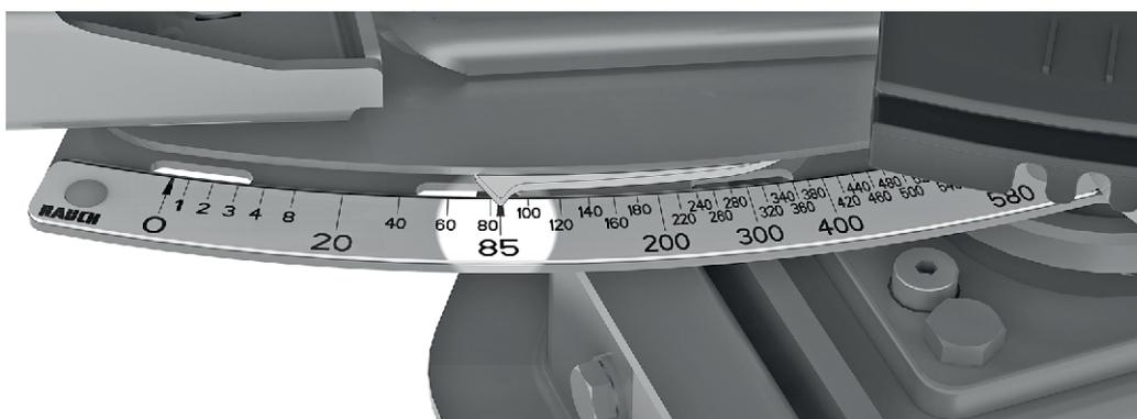
*Fig. 89: Metering slide pointer on scale value 85*
