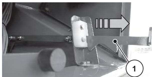
Fig. 55: Cleaning flap lever
