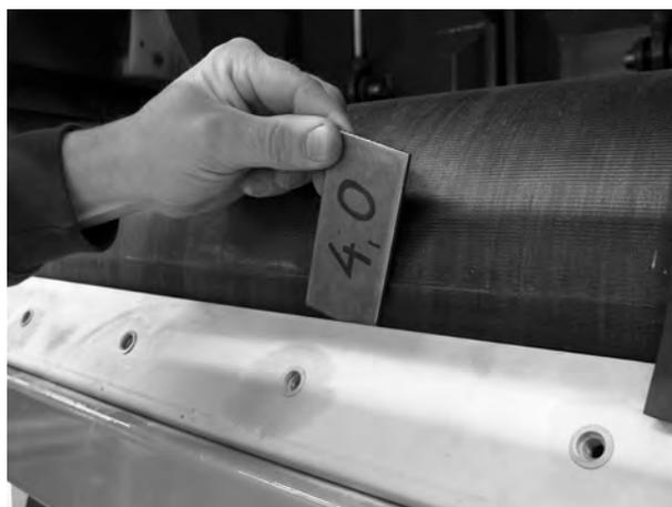
Fig. 129: Checking the clearance
