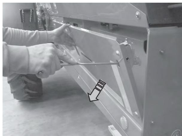
Fig. 89: Folding open the side cover
