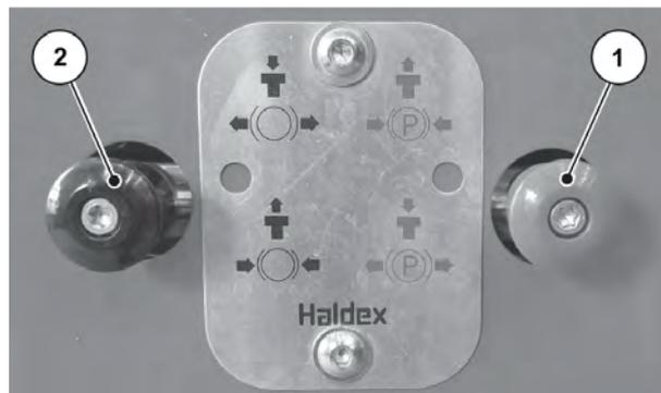
*Fig. 33: Disengaging the parking brake*
