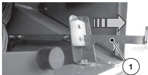
*Fig. 91: Cleaning flap lever*
