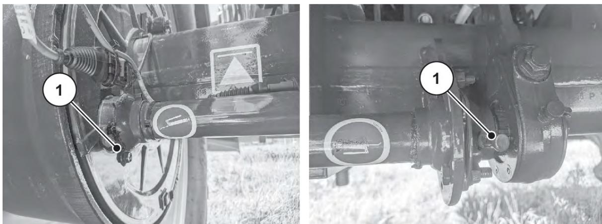
Fig. 99: Rigid axle brake camshaft bearing
