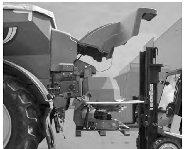
Fig. 46: Positioning the forklift truck
