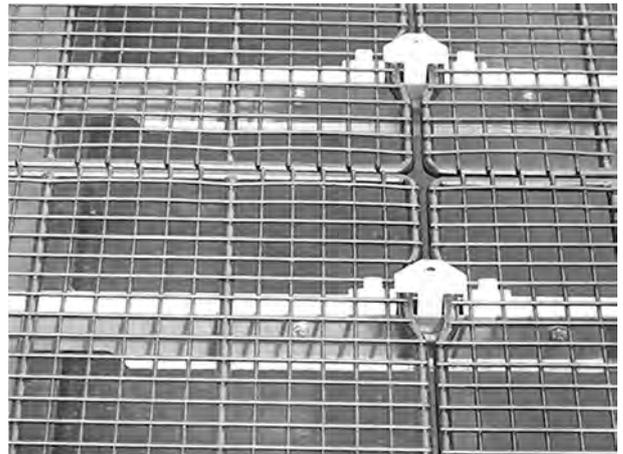
*Fig. 44: Feeder mesh in hopper*
