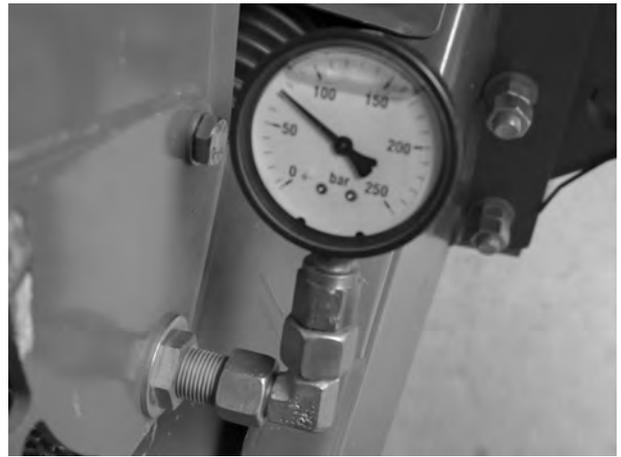
*Fig. 122: Pressure gage at cable guide via towing bar*
