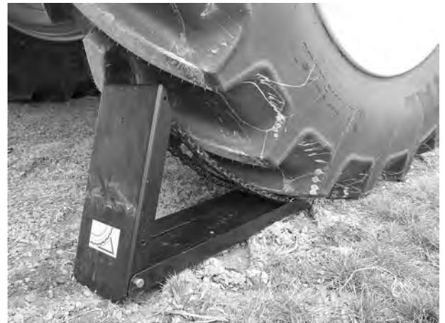
Fig. 82: Positioning the wheel chock
