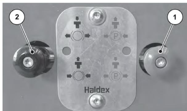
*Fig. 80: Engaging the manual parking brake*
