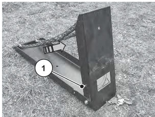
Fig. 85: Fold out the wheel chock
