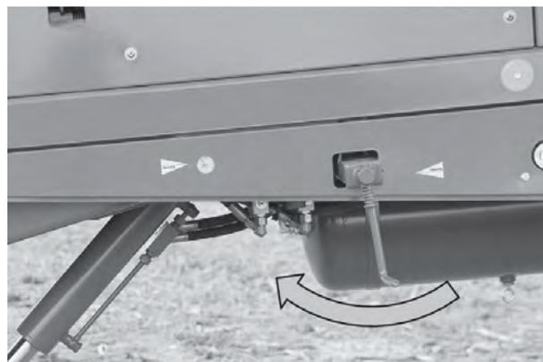
Fig. 84: Engaging the manual parking brake
