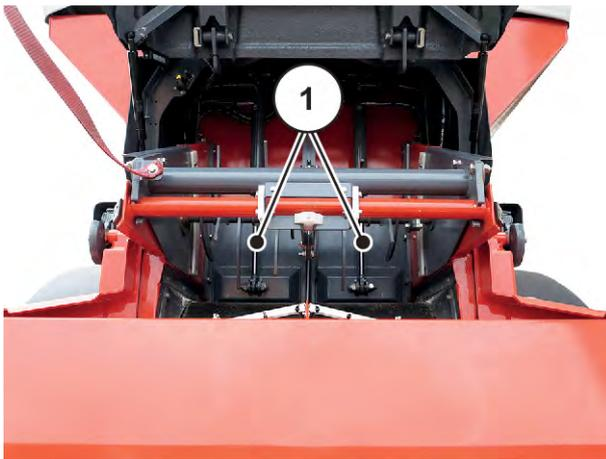
Fig. 52: Pre-metering slide in closed position
