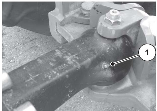
[1] Lubrication point: ball coupling
