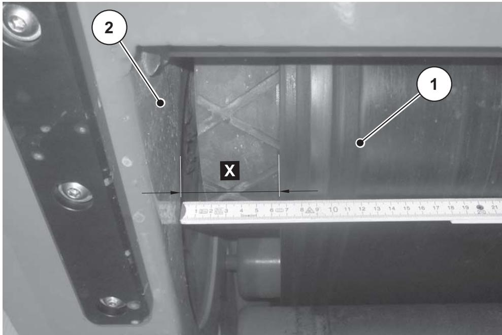
**Figure 9.15:** Inspection of the conveyor belt position
