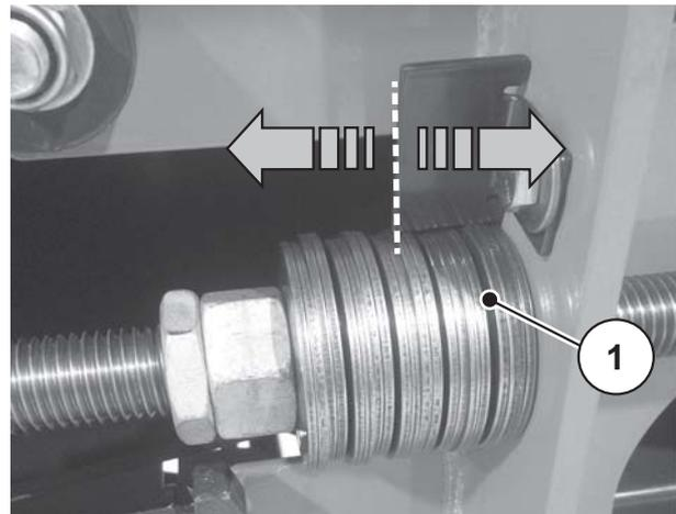
**Figure 9.19:** Adjusting the disc spring packages
