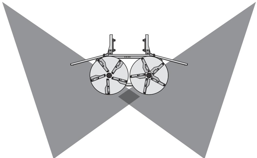
**Figure 7.18:** Insufficient lime in the middle
