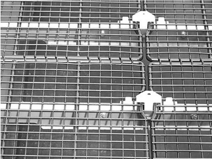
**Figure 6.26:** Securing the feeder mesh in the hopper
