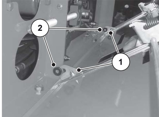
Figure 9.4: Fitting the side cover
