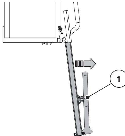
**Figure 6.38:** Unfolding the bottom part of the ladder
