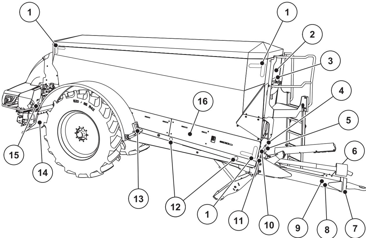
**Figure 3.2:** Position of the safety equipment, warnings and instructions, side view
