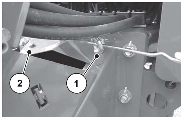
**Figure 6.1:** Removing the protective plate
