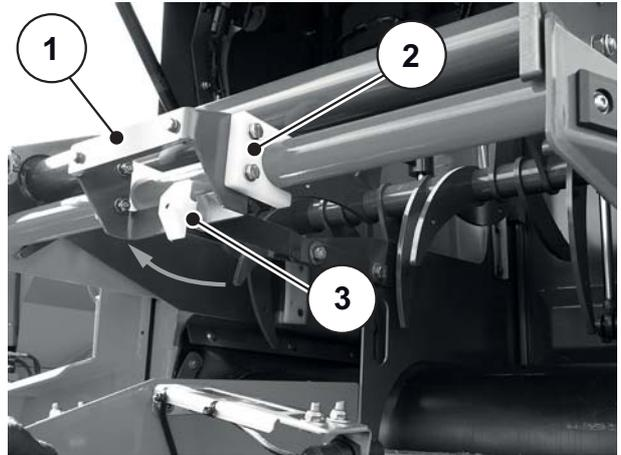
**Figure 6.21:** Securing the separating plate
