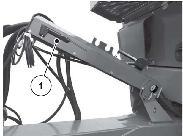
[1] Adjustment lever (left in direction of travel, hose storage place)
