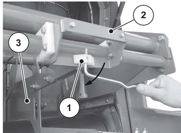
**Figure 6.18:** Removing the separating plate
