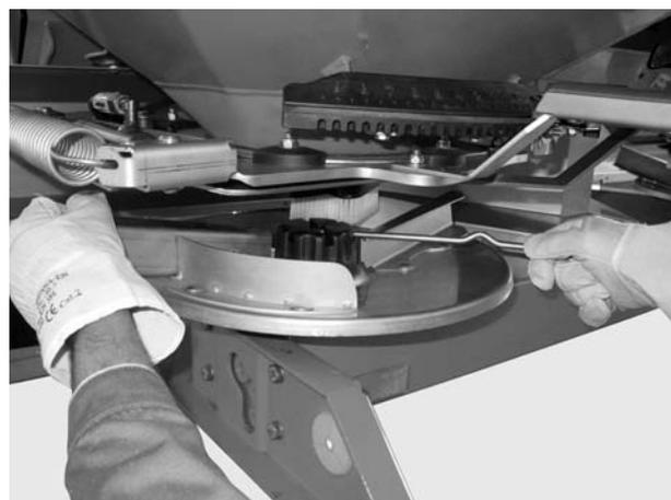
**Figure 7.8:** Undoing the cap nut
