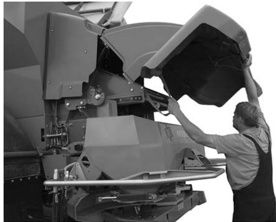
**Figure 7.2:** Pulling the tieback
