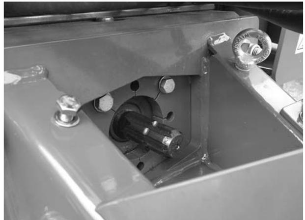
**Figure 6.2:** Greasing the gear journal
