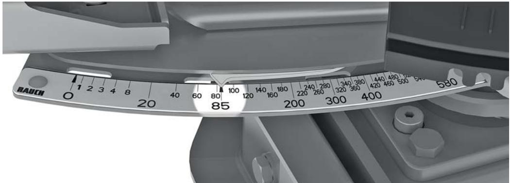
**Figure 7.11:** Scale for displaying the spreading quantity
