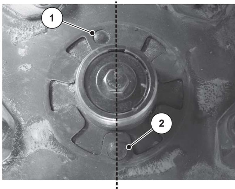
**Figure 9.9:** Distinguishing the side of the spreading discs
