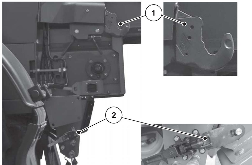
**Figure 6.27:** Coupling points on the AXENT 100.1
