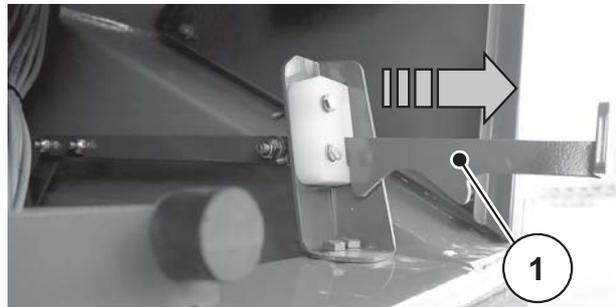
Figure 9.5: Lever of the cleaning flap
