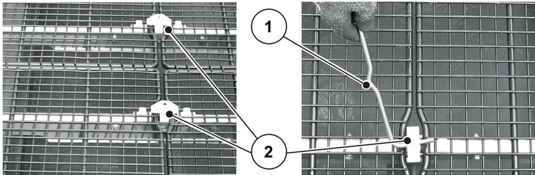
**Figure 6.16:** Unlocking the holders
