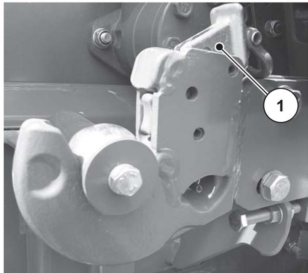
**Figure 6.33:** Securing the spreading unit at the bottom
