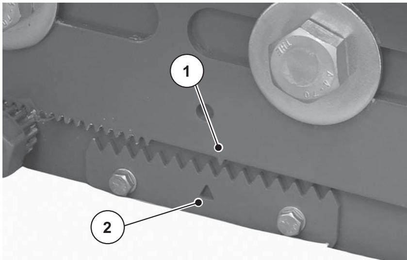
**Figure 7.16:** Drop point in neutral position
