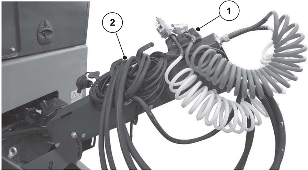
**Figure 7.24:** Storage console for cables, hydraulic hoses and pneumatic lines
