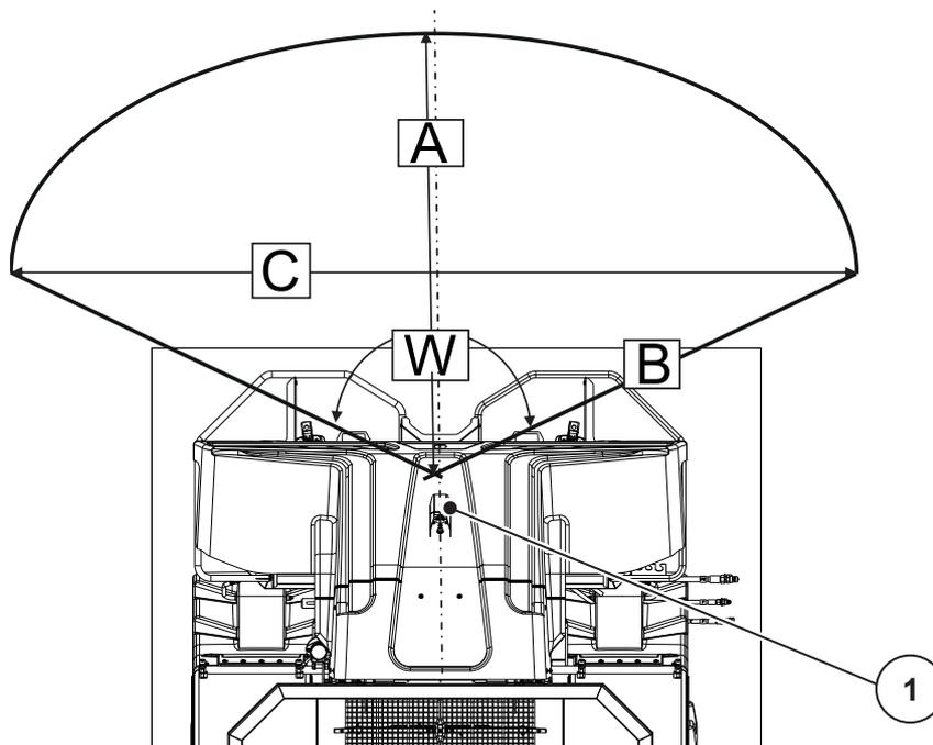
**Figure 6.41:** Field of vision of rear view camera
