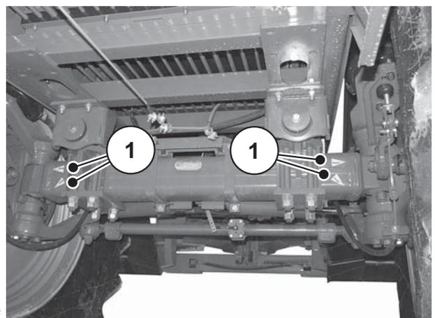
[1] Lubrication point: brake linkage
