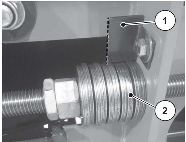
**Figure 9.17:** Re-tightening the disc spring packages
