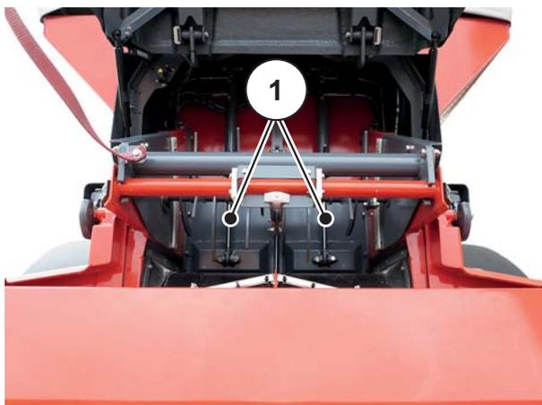
**Figure 6.34:** Pre-metering sliders in closed position
