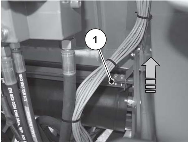
**Figure 6.35:** Cleaning flap in closed position, at the front in the direction of travel
