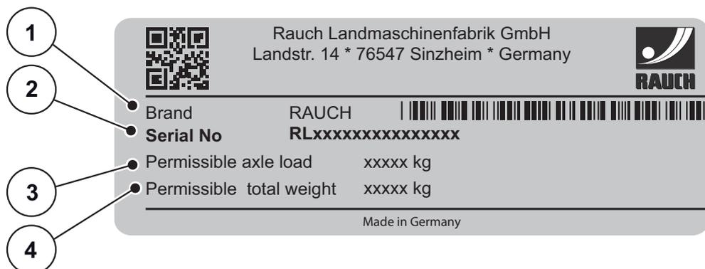
Figure 3.7: 2. Nameplate for towed machines
