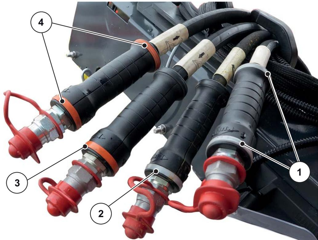
**Figure 6.7:** Identification of the hydraulic hoses
