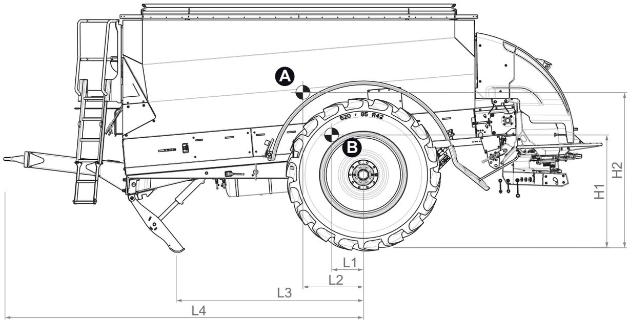
**Figure 4.7:** Centre of gravity in top hitching
