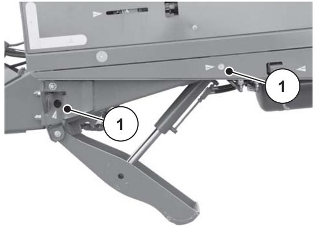
[1] Lubrication points: towing bar
