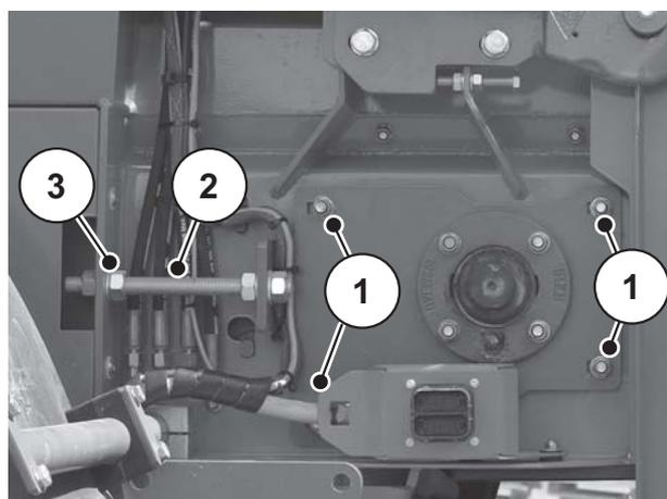
**Figure 9.16:** Position of the drive roller
