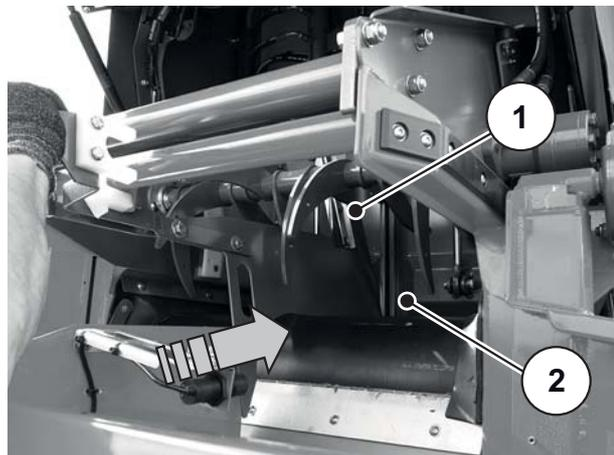
Figure 6.19: Installing the separating plate
