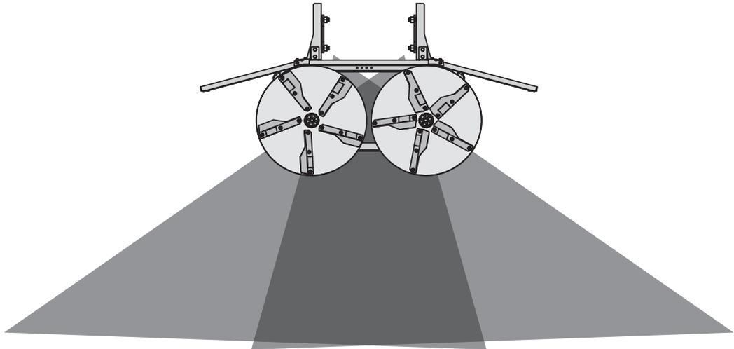
**Figure 7.19:** Excessive lime in the middle
