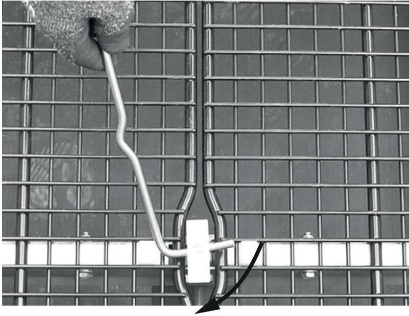
**Figure 6.25:** Locking the feeder mesh
