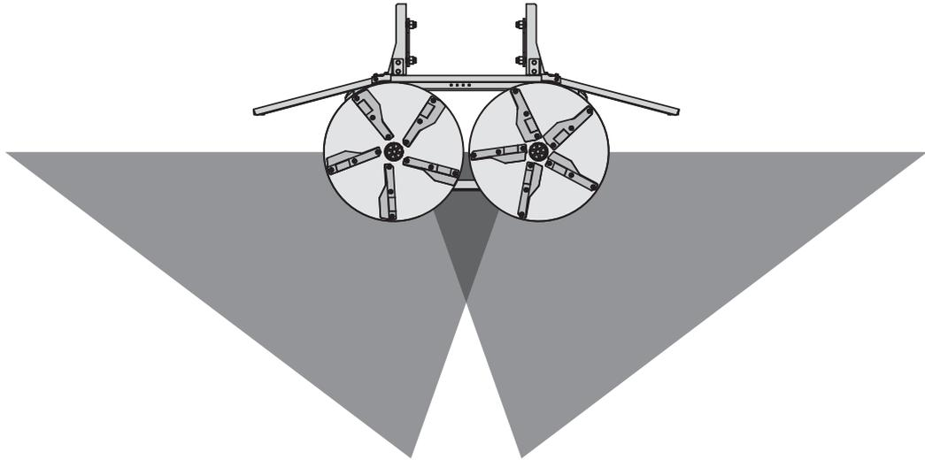
**Figure 7.15:** Normal spreading pattern, drop point in neutral position
