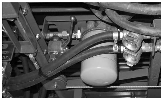
Figure 9.28: Oil filter, towing bar suspension
