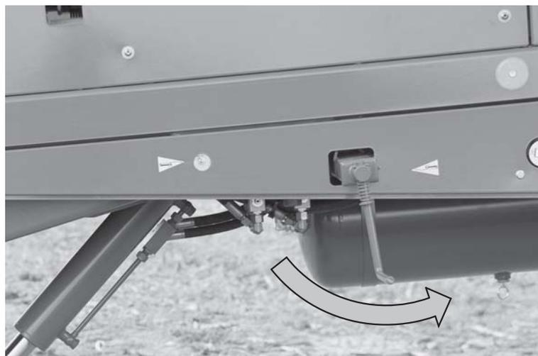
**Figure 6.14:** Releasing the manual parking brake
