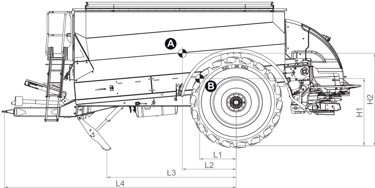
**Figure 4.6:** Centre of gravity in bottom hitching
