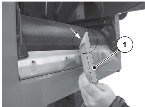
**Figure 9.23:** Applying the clamping plate
