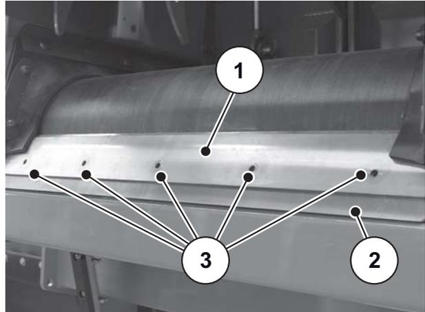
Figure 9.20: Dismantling the clamping plate
