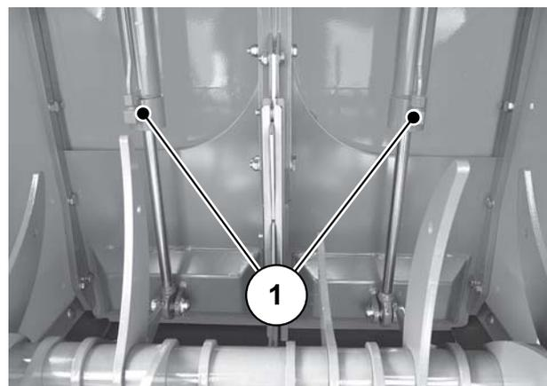
Actuating functions: hydraulic cylinders [1] of the pre-metering sliders.
