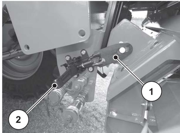
**Figure 6.32:** Securing the spreading unit at the bottom
