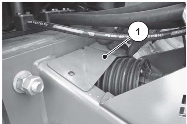
**Figure 6.4:** Fitting the protective plate
