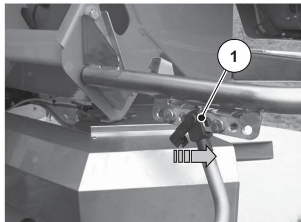
**Figure 6.31:** Fastening the mudguard extension
