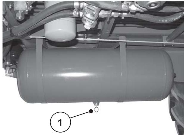
**Figure 9.24:** Draining the air tank
