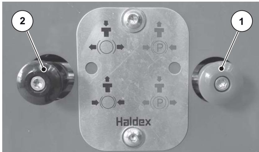
**Figure 6.13:** Releasing the parking brake
