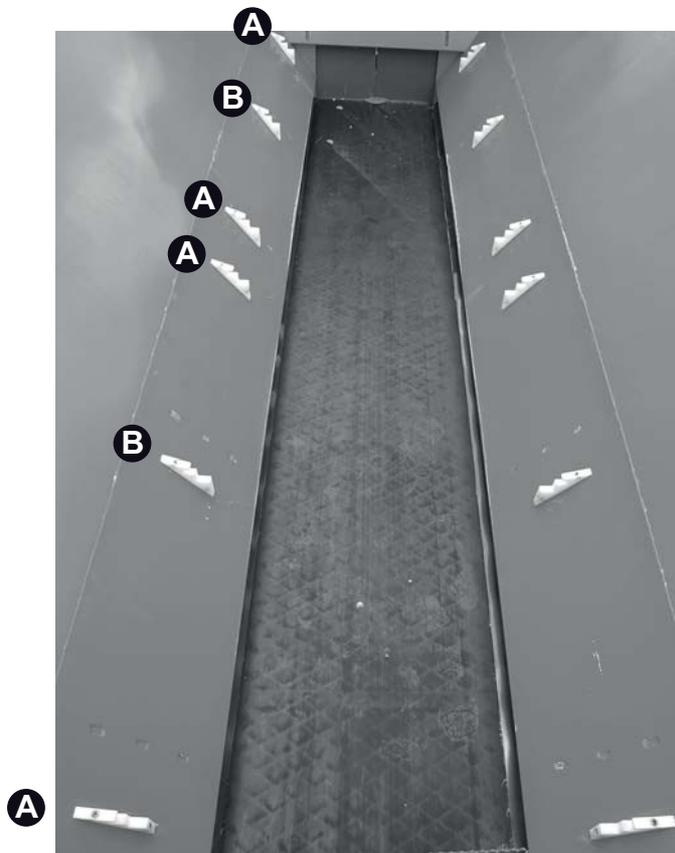
**Figure 6.23:** Installing the holders of the feeder mesh
