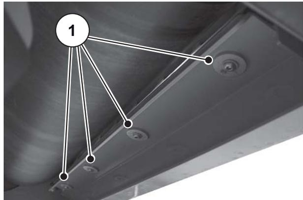
**Figure 9.22:** Adjusting the position of the holder
