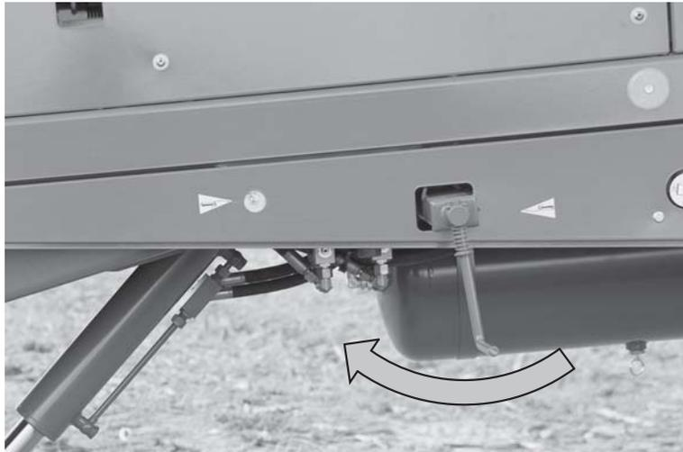
**Figure 7.21:** Applying the manual parking brake
