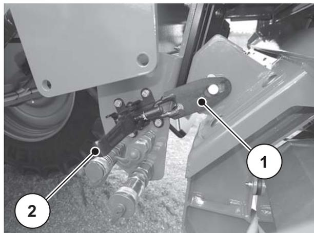
**Figure 6.29:** Securing the spreading unit at the bottom
