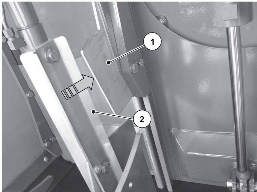
Figure 6.20: Inserting the separating plate in guides
