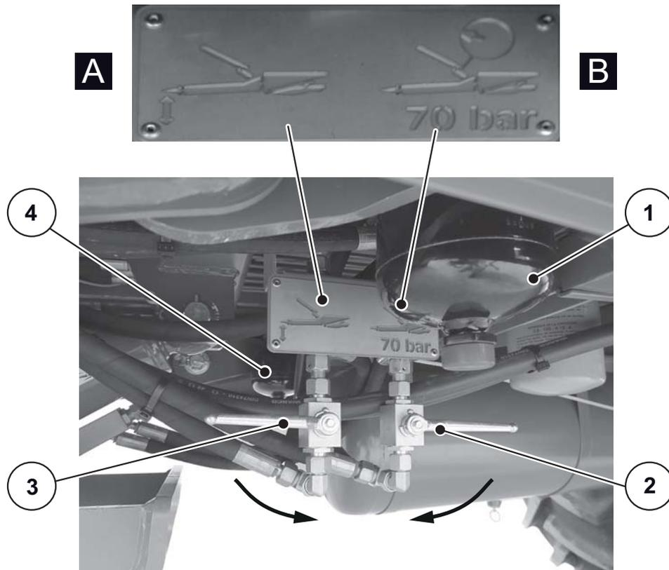
**Figure 9.10:** Setting the towing bar suspension
