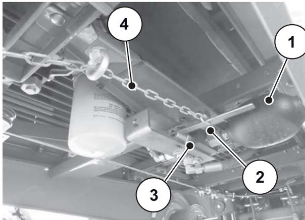
**Figure 6.12:** Breakaway coupling of the hydraulic brake system
