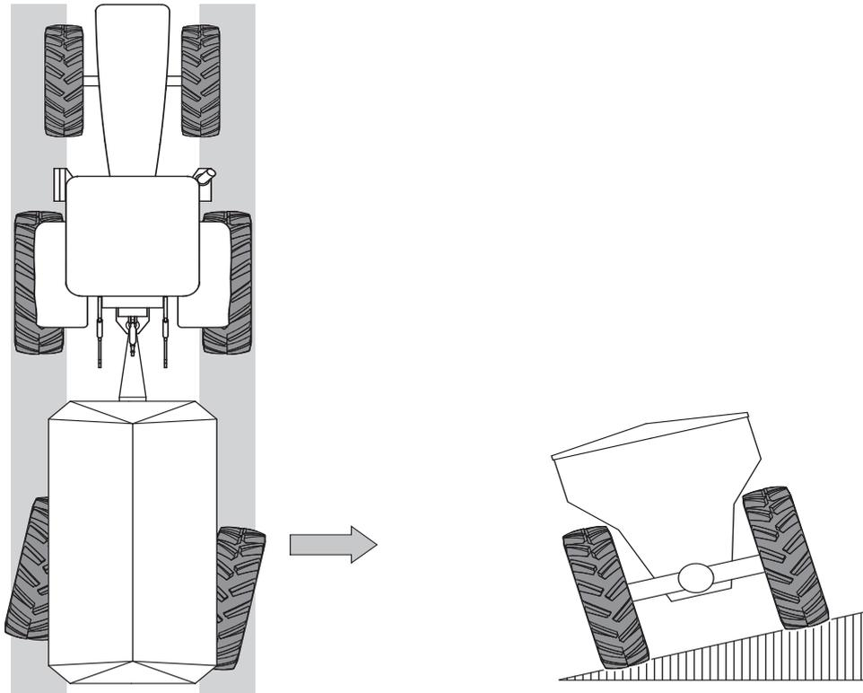
**Figure 7.14:** Kingpin steering (special equipment)
