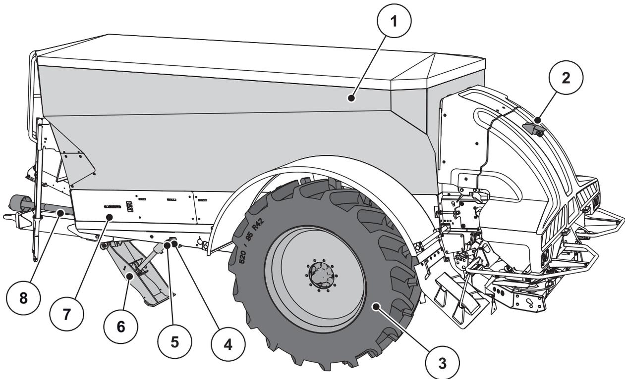
**Figure 4.1:** Assemblies and function of the machine AXENT, side view
