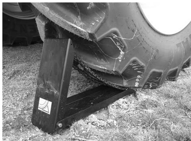
**Figure 7.23:** Positioning a wheel chock
