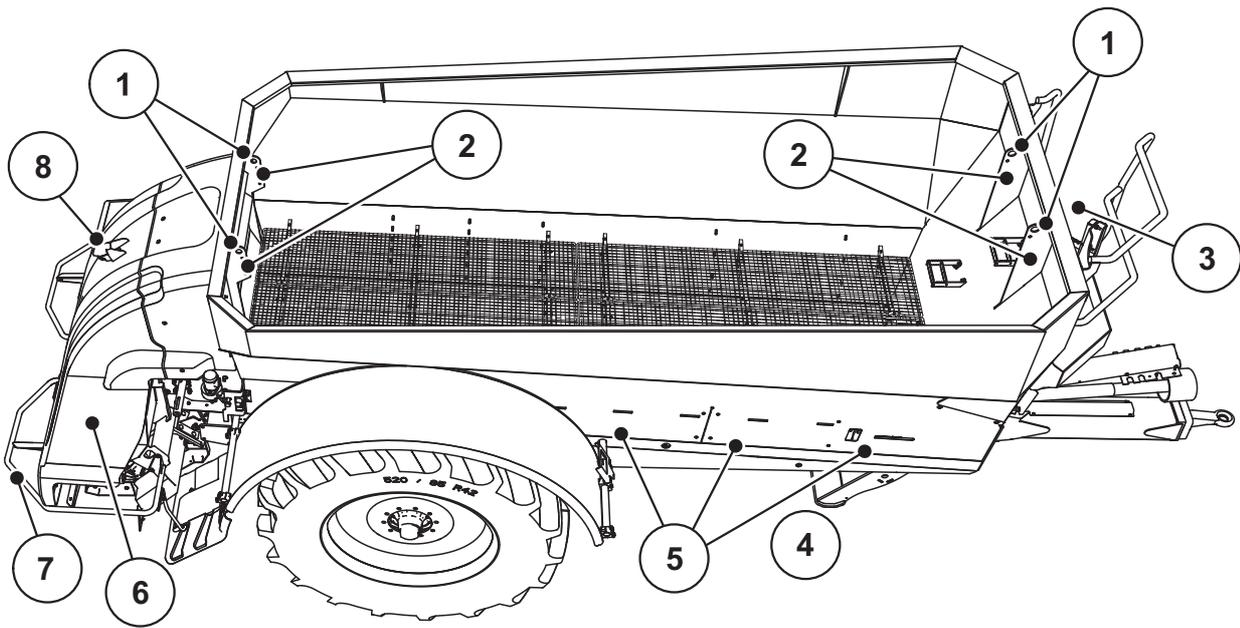
**Figure 3.4:** Position of the safety equipment, warnings and instructions, top
