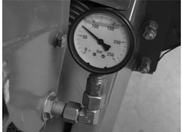
**Figure 9.14:** Pressure gauge at cable guide above towing bar
