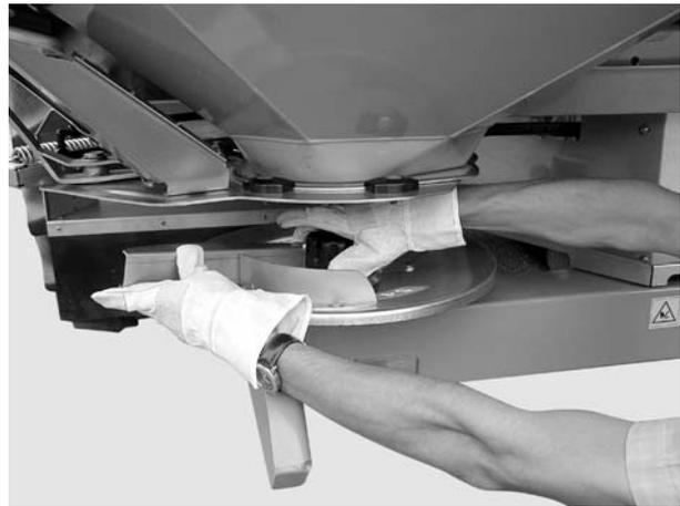
**Figure 7.9:** Unscrewing the cap nut
