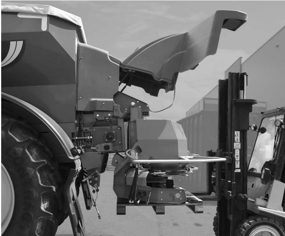
**Figure 6.28:** Approaching with the forklift
