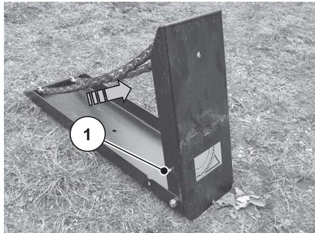
**Figure 7.22:** Opening a wheel chock
