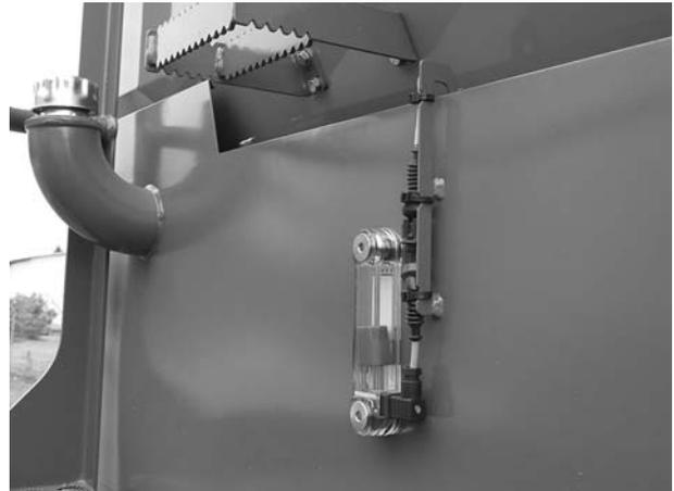
**Figure 9.25:** Oil level indicator position
