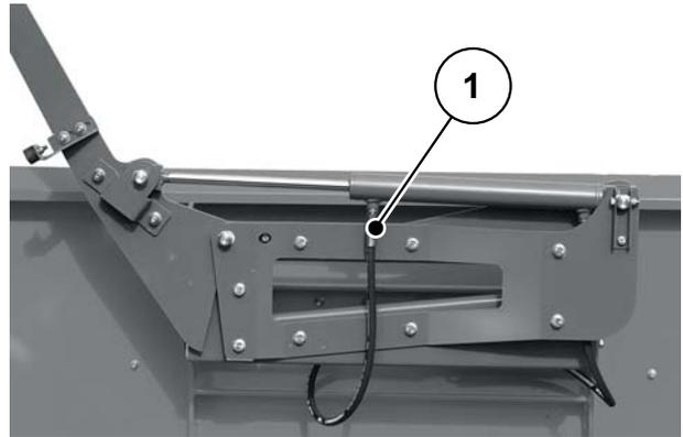
**Figure 9.32:** Hydraulic cylinder, hopper cover
