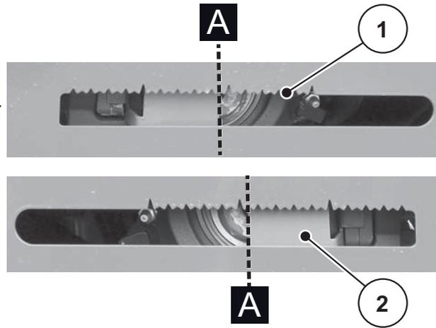
**Figure 9.18:** Setting the disc spring packages
