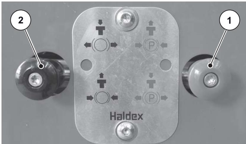
**Figure 7.20:** Releasing the manual parking brake
