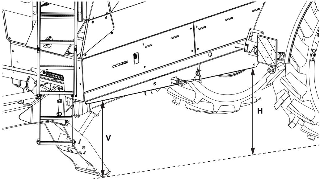
**Figure 9.11:** Checking the machine inclination
