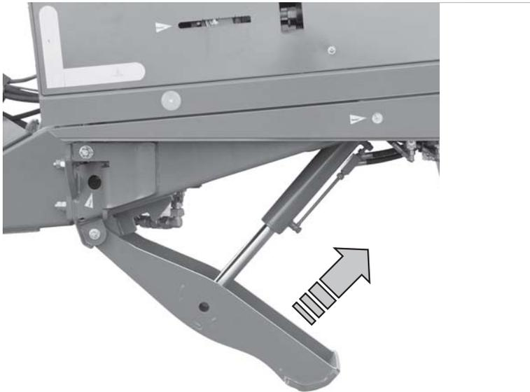
**Figure 6.8:** Retracting the support stand
