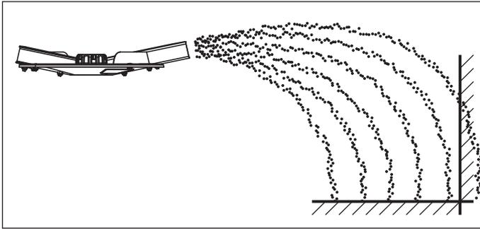
**Figure 7.6:** Full border spreading with normal fertilisation
