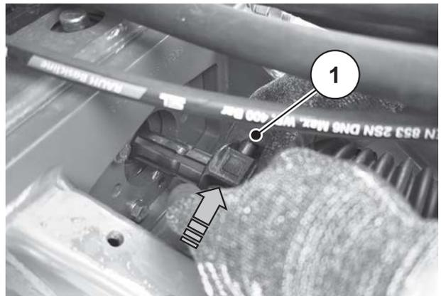
**Figure 6.3:** Fitting the universal drive shaft on the gear journal
