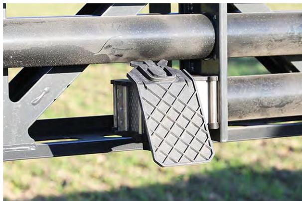
Fig. 46: Baffle in normal fertilizing mode
