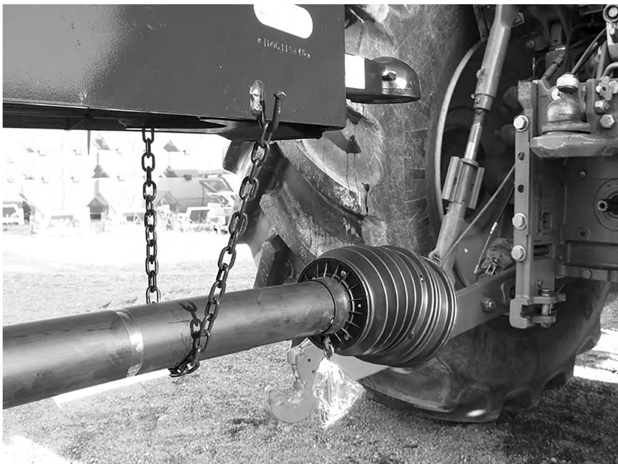
Fig. 24: Storing the universal drive shaft
