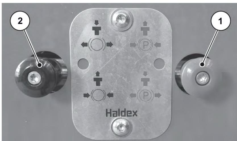
Fig. 43: Disengaging the parking brake
