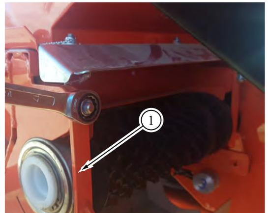
Since the metering rollers are often seated very tightly in the bracket, it is possible to insert a mounting lever or a shaft into the metering roller and use it to pry it out for easier removal.
