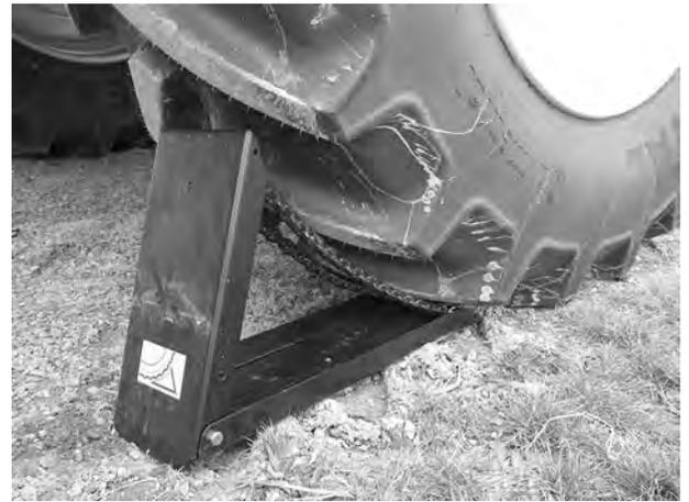
Fig. 55: Positioning the wheel chock
