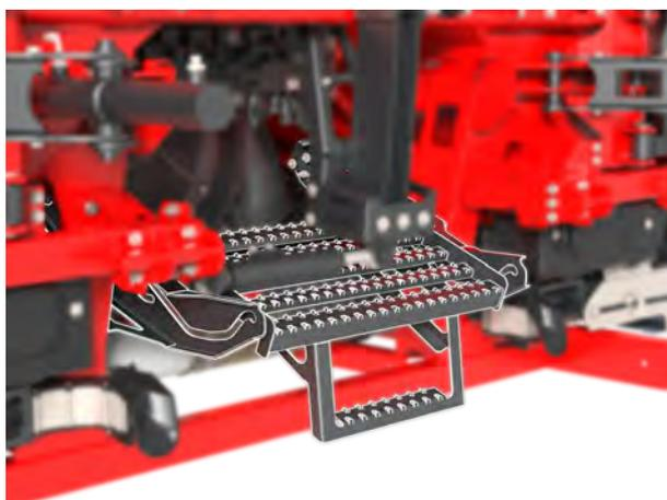
*Fig. 26: Step retracted*
