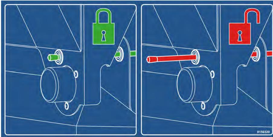
Fig. 39: Locking mechanism display
