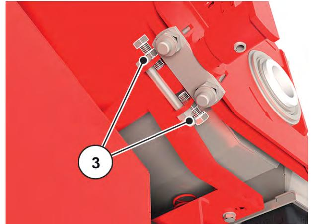
Fig. 61: Setting the distance between the cam wheels and the spreader tank
