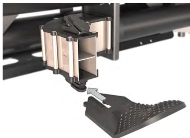
*Fig. 46: Switching the baffle*
