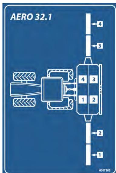
Fig. 29: Illustration of the sections on the boom-type mineral fertilizer spreader
