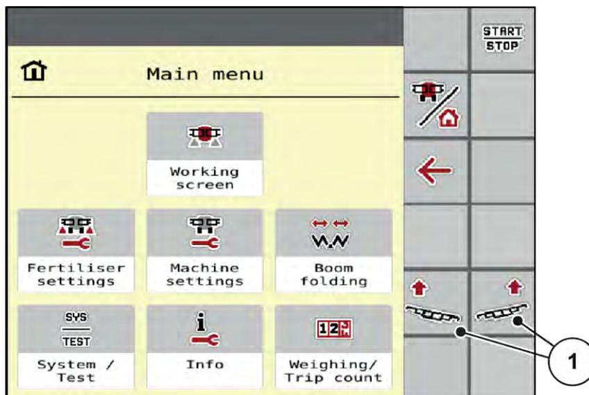
Fig. 43: Function keys for adjusting the boom inclination
