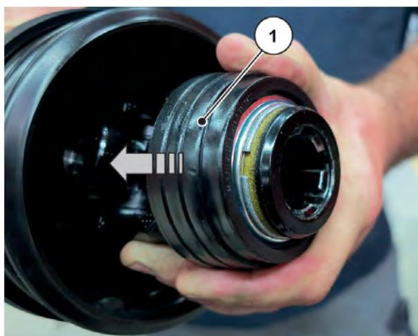
Fig. 21: Pulling back the pulling sleeve
