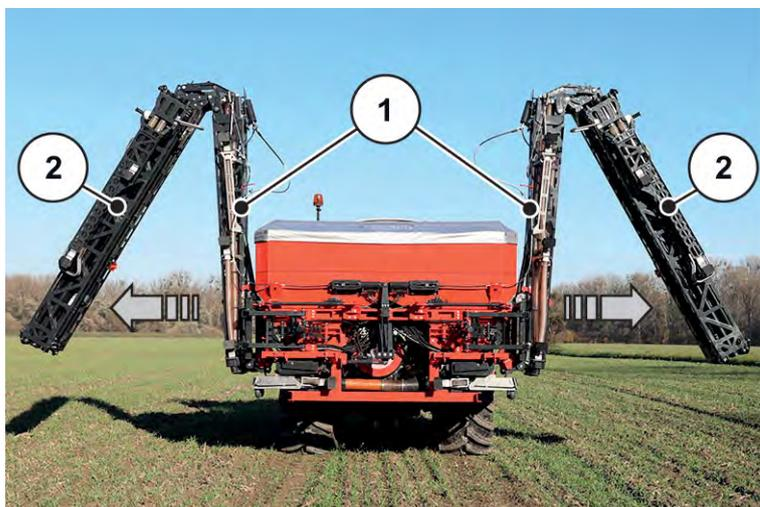
Fig. 42: Swinging out the start sections and central sections 1
