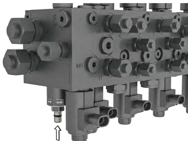
Fig. 13: Position of the LS/CC valve
