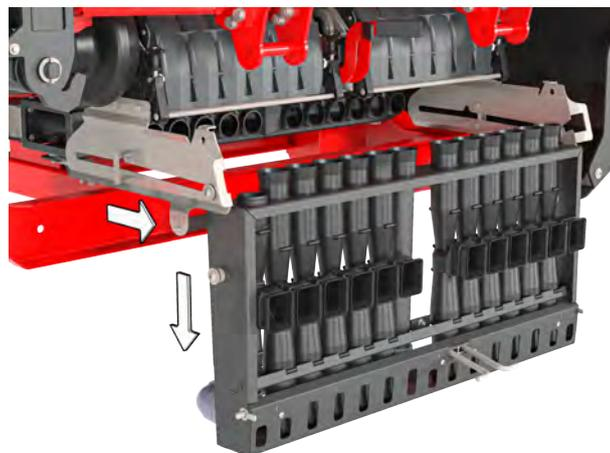
Fig. 31: Lowering the injector cartridge
