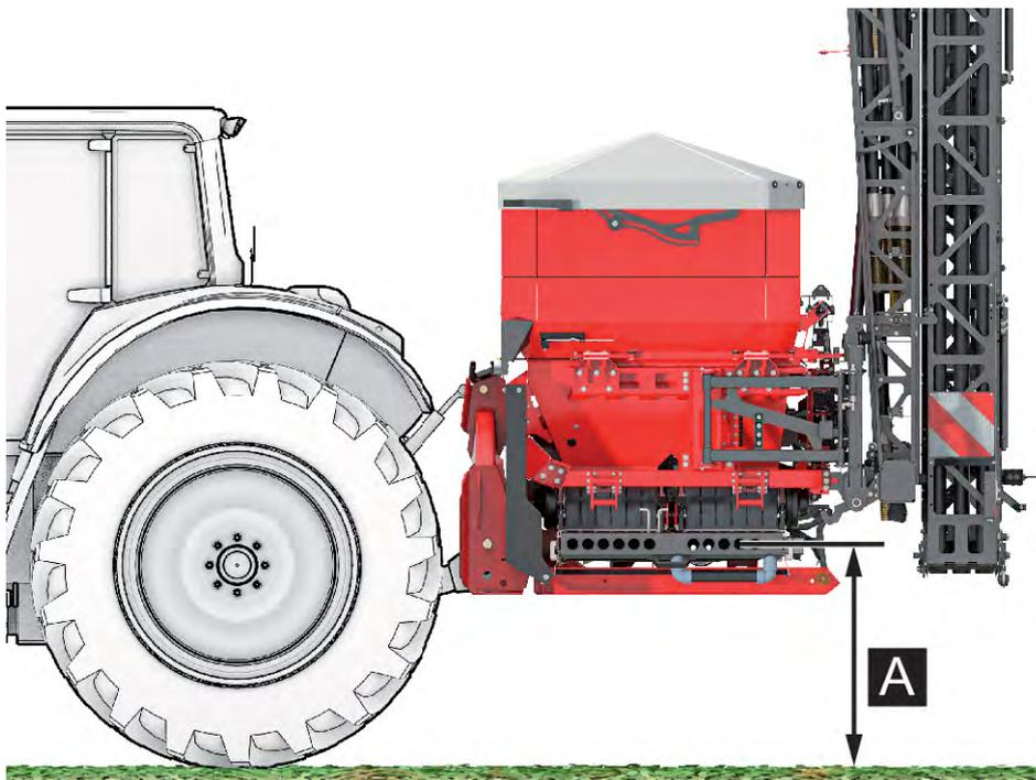
Fig. 25: Ideal mounting height for normal and late fertilizing
