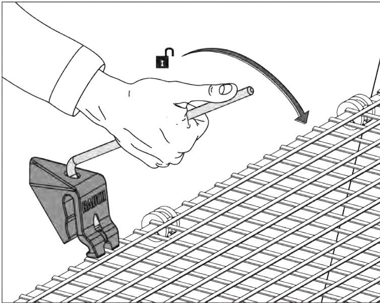
Fig. 57: Opening the protective grid lock
