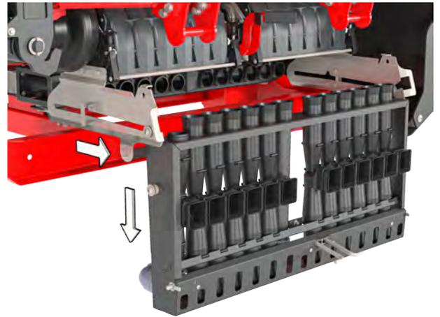
Fig. 50: Lowering the injector cartridge
