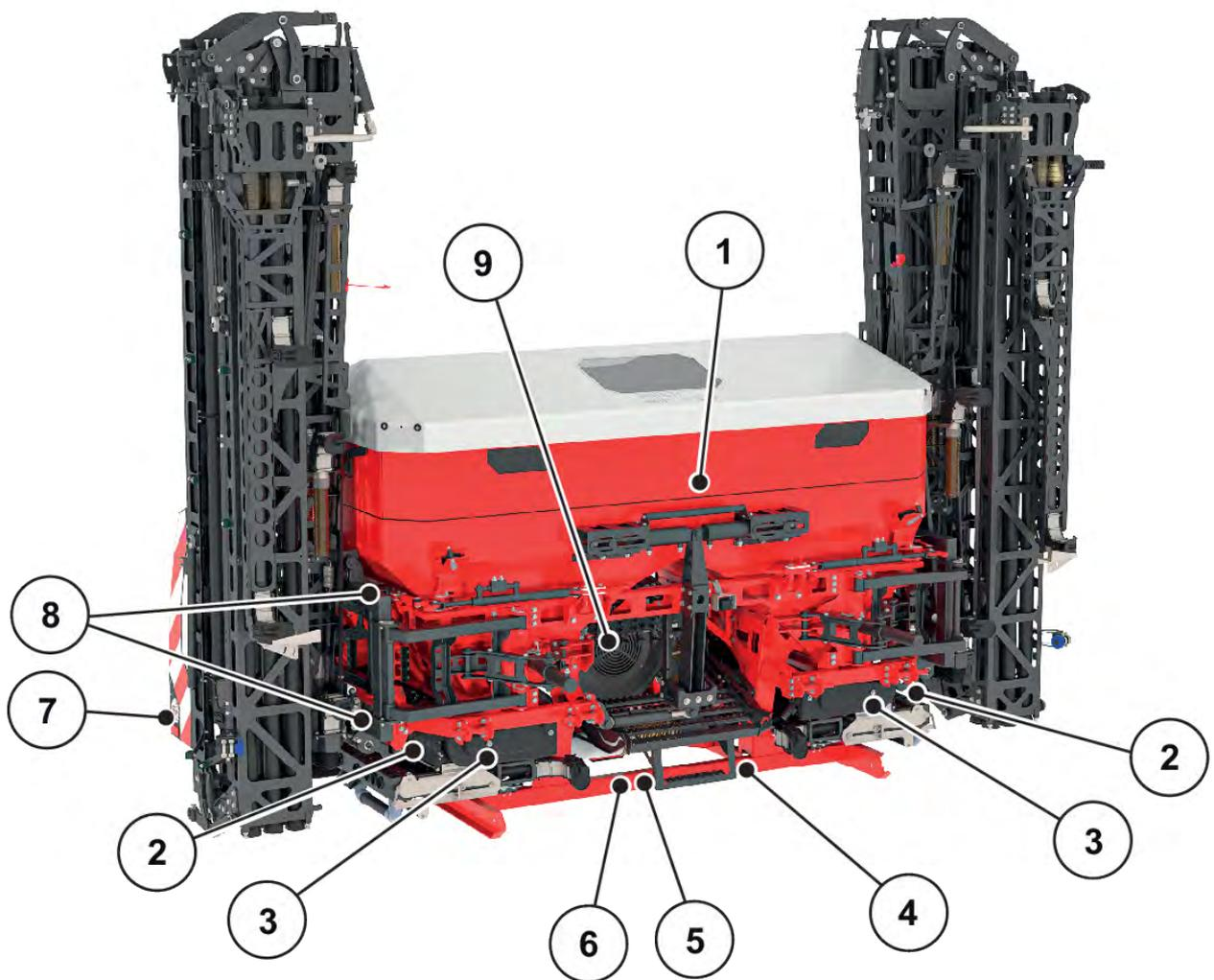
*Fig. 3: Safety equipment, warning and instruction stickers, rear*
