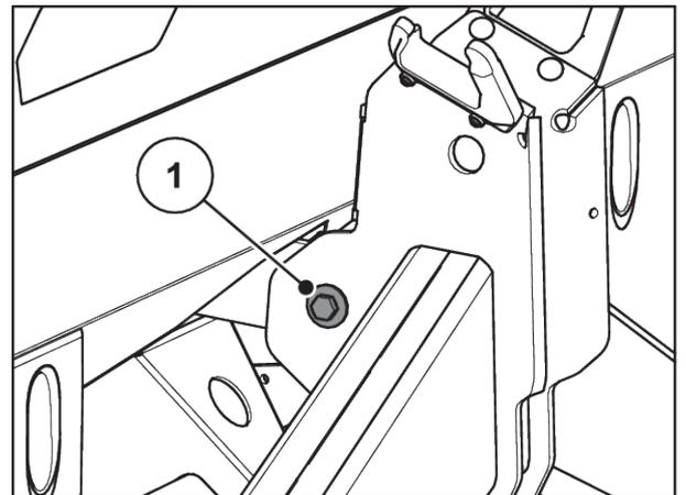
*Fig. 55: Fastening the tie rod at the weigh frame*
