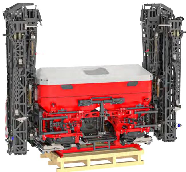
Fig. 53: Placing the machine on a pallet
