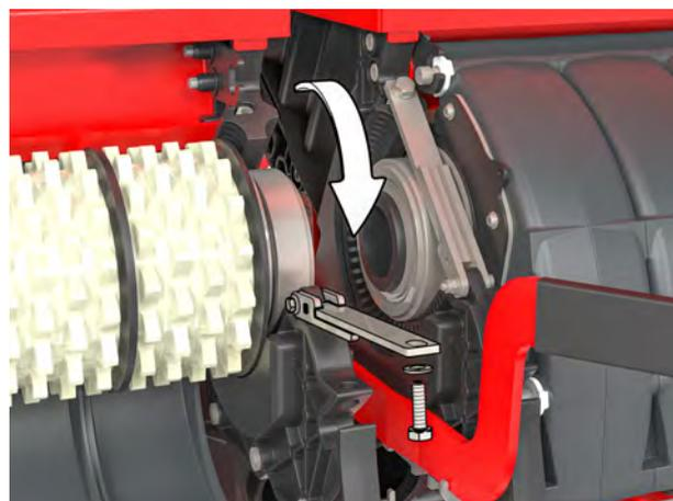
*Fig. 38: Opening the metering roller bracket*
