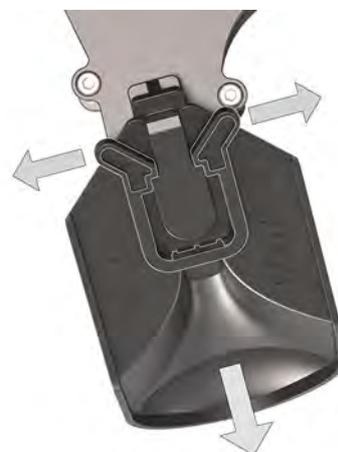
*Fig. 45: Pulling out the baffle*
