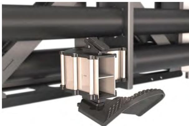
Fig. 47: Baffle in late fertilizing mode
