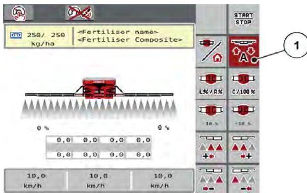
Fig. 20: DistanceControl button enabled
