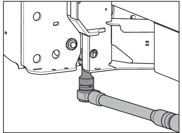
*Fig. 54: Fastening the weigh cells (on the left side of the direction of travel)*
