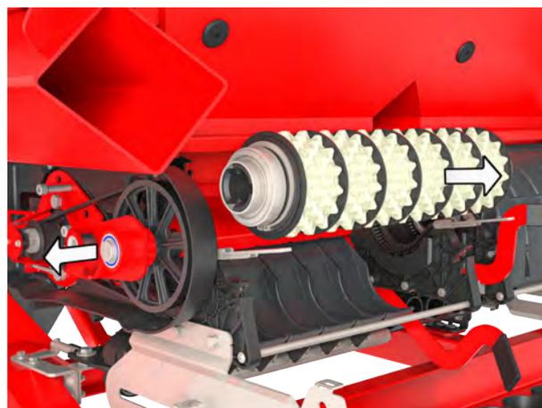
The metering roller can be installed by following the same steps for removal in the reverse order.
