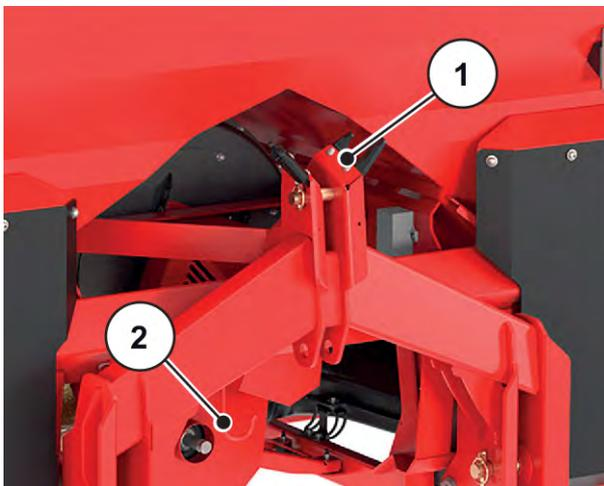
Fig. 23: Storage of the cables and hydraulic hoses
