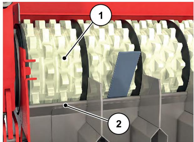
*Fig. 60: Checking the distance between the cam wheels and the spreader tank*
