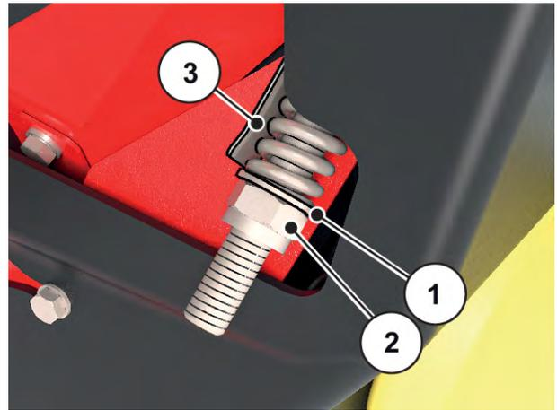
*Fig. 62: Blower belt tensioning mechanism*
