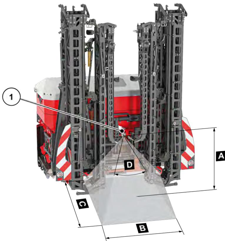
Fig. 14: Rear view camera field of vision when in transport position
