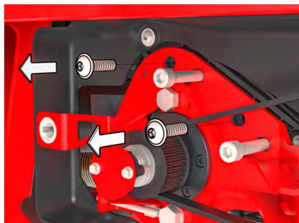
*Fig. 37: Releasing screws on the motor*
