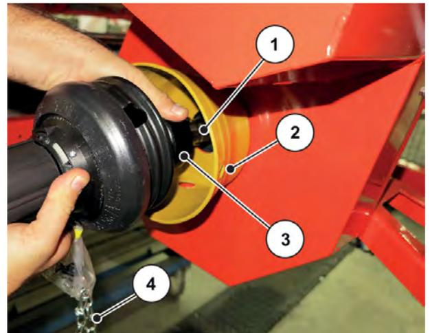
Fig. 22: Securing the universal drive shaft
