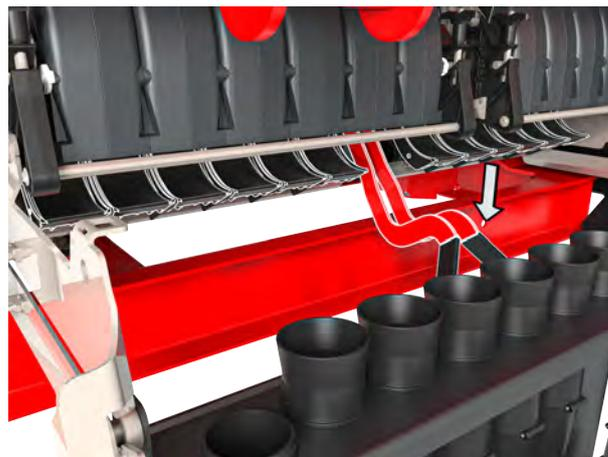
*Fig. 51: Opening the locking mechanism of the metering tank*
