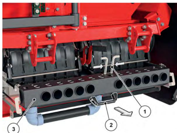
Fig. 49: Unlocking the injector cartridge
