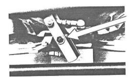
Lubricate this grease nipple after every cleaning operation.
